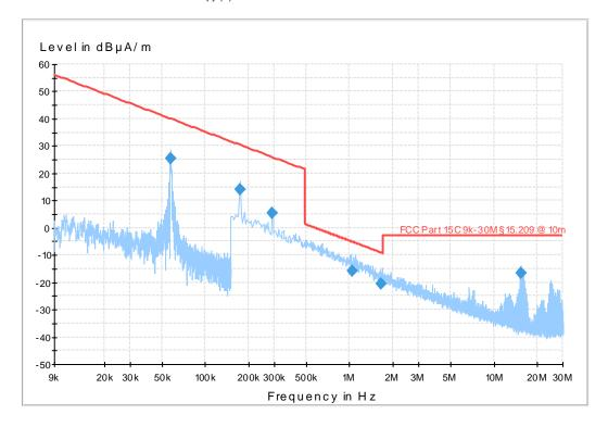
Magnetic field strength preview, max peak at a distance of 10 m, antenna in z-position Copy (2) of Radio EN300330 H-field 9kHz - 30MHz
