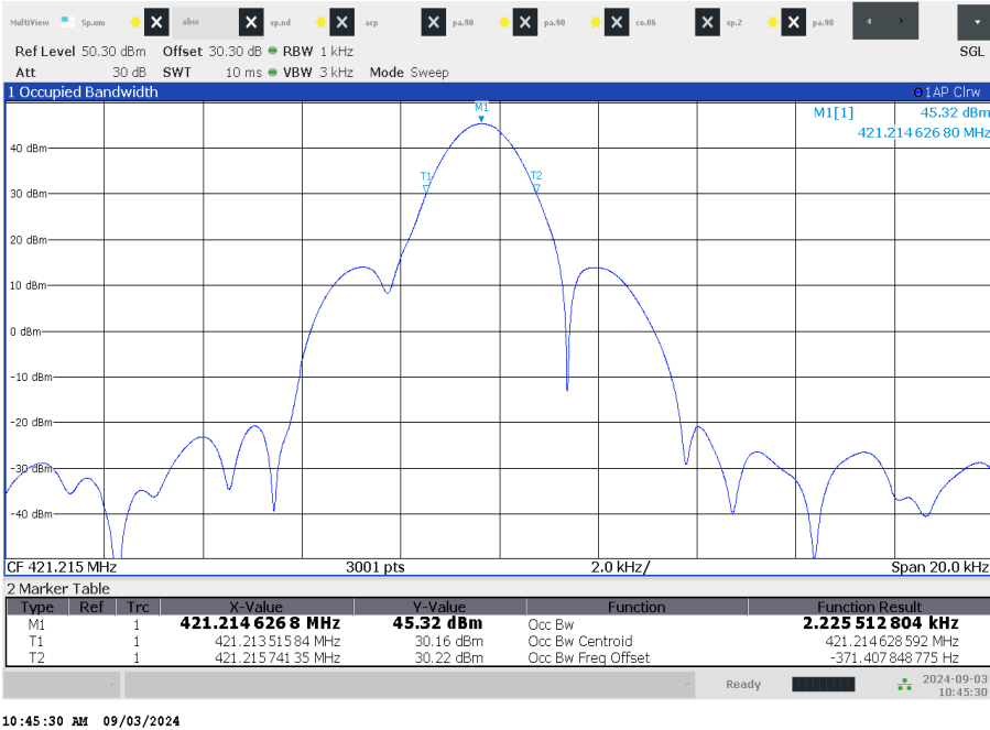
Plot 7: 421.2125 MHz / 4800 bits per second, 1 kHz RBW
