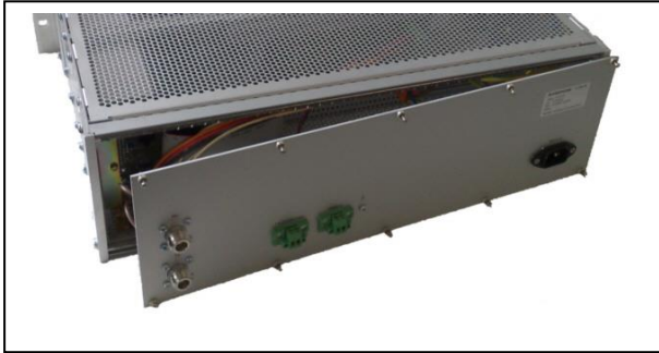
Figure 9: Removing the back panel from the ITC2500-NA
