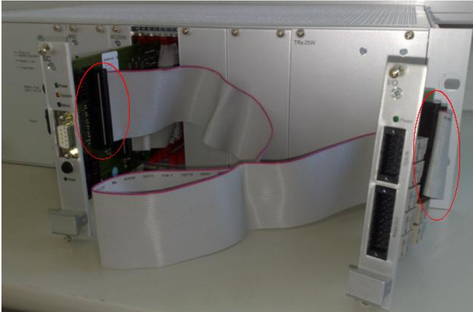
Figure 15: Connecting the I/O card to the ITC2500-NA
