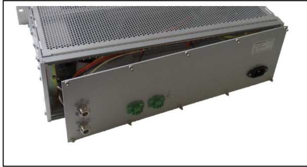
Figure 17: Removing the back panel from the ITC2500-NA
