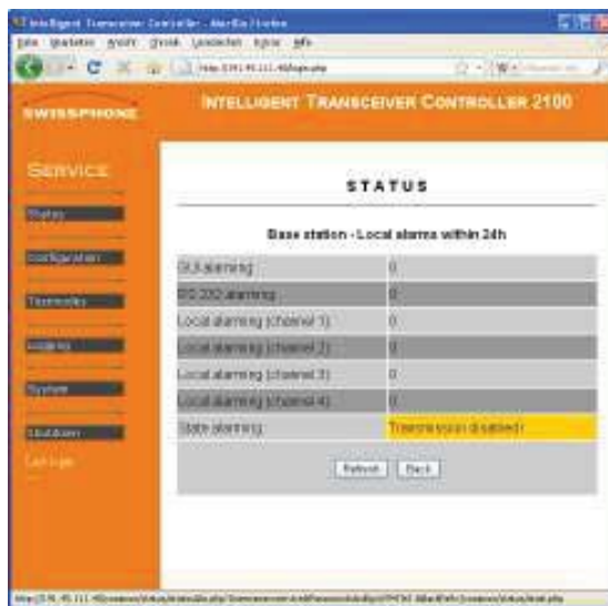
Fig. 7-17: Disabled transmission when the serial interface is used for a local task
