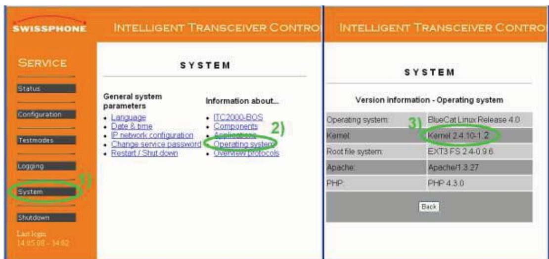
Fig. 9-5: Checking the kernel version
