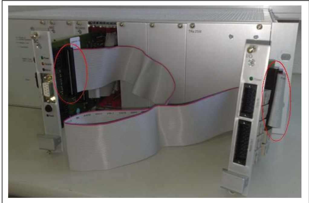
Fig. 6-11: Connection of the I/O to the ITC2100-BOS
