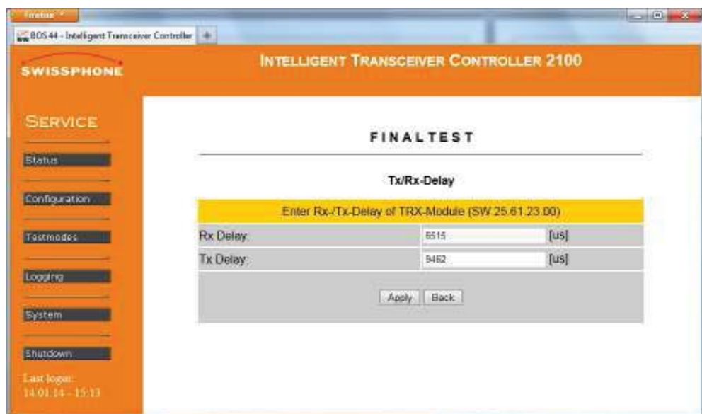
Fig 9-3: Enter the Rx/Tx delay values of the new transceiver module
