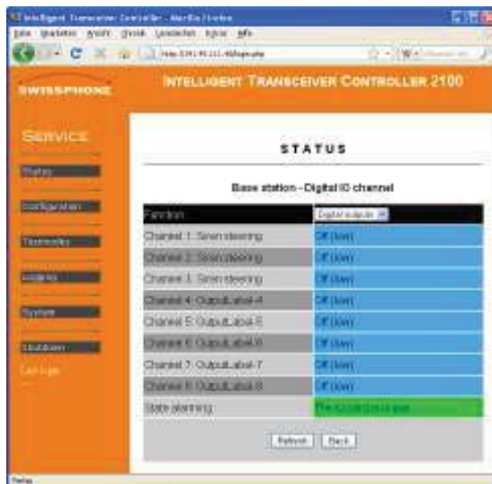
Fig. 7-15: Status of the digital outputs at activated siren control
