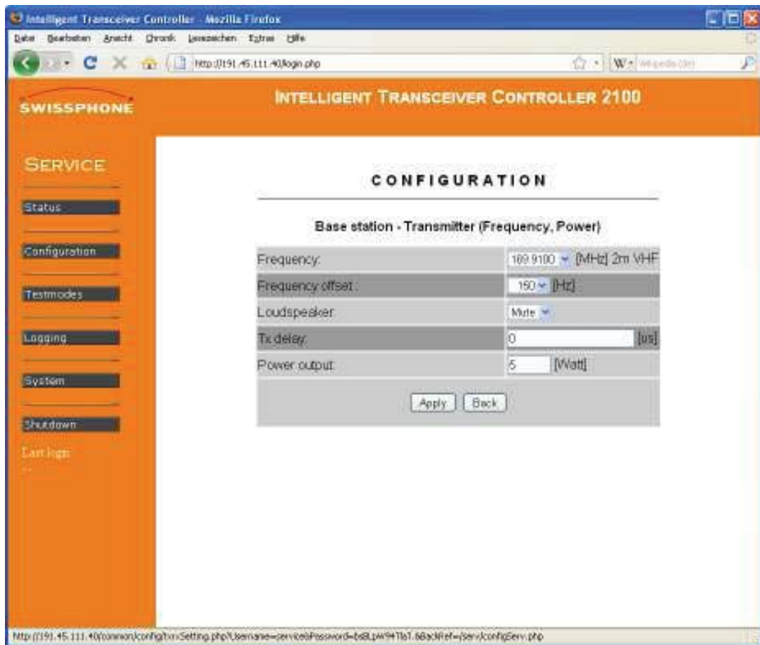
Fig. 7-30: Configuration of the transmitter parameters
