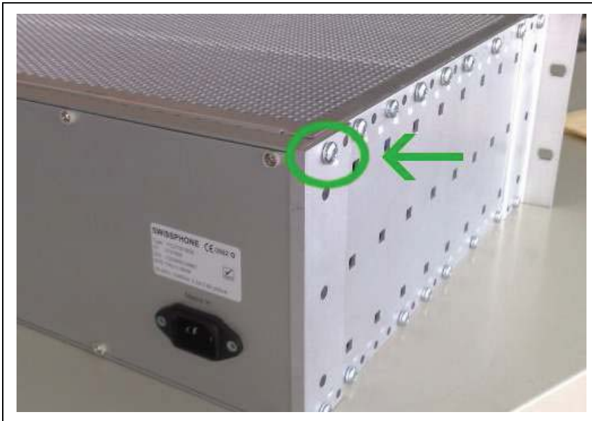
Fig. 6-1: Grounding point at ITC2100-BOS
