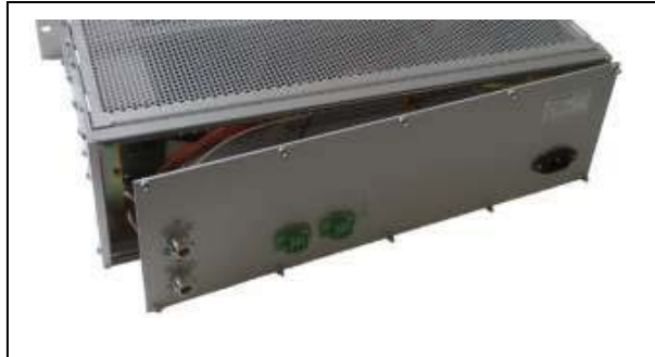
Fig. 6-4: Removing the ITC2100-BOS back panel
