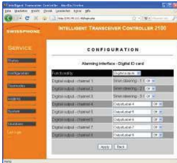
Fig. 7-26: Configuration of the digital outputs at activated siren control
