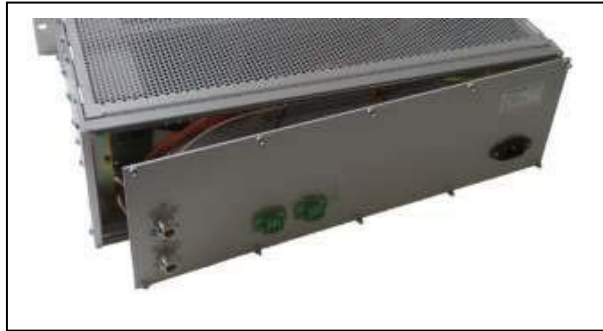
Fig. 6-13: Removing the ITC2100-BOS rear panel
