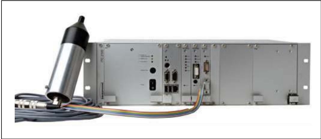
Fig. 6-7: Connection of GPS antenna to Master-ITC
