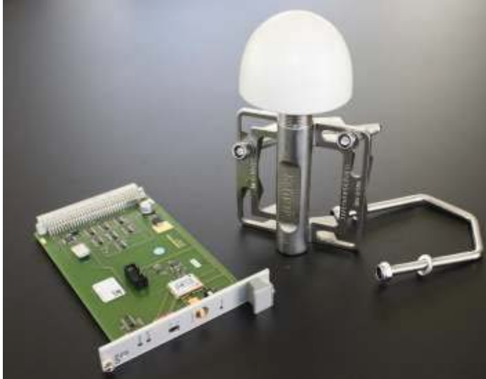
Fig. 6-8: GPS receiver card with potential GPS antenna and fixture
