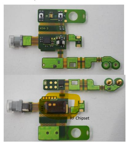
Antenna internal picture (antenna PCB is externally sourced and there are no components on it)
