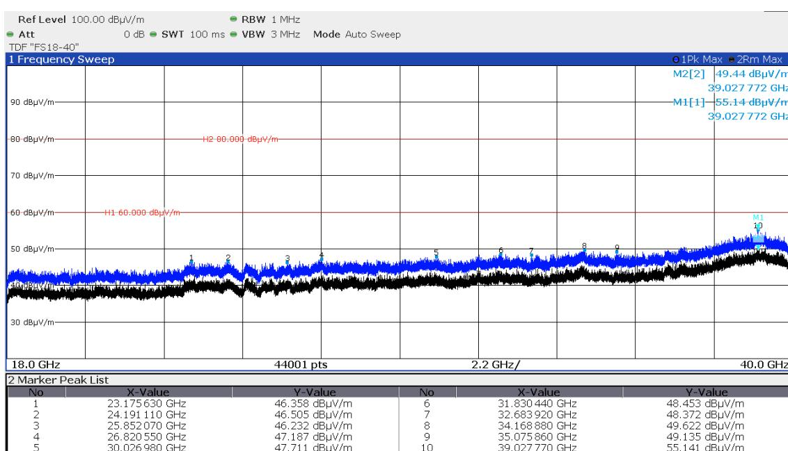
Result: Exempt for the UWB transmission, the radiated emissions are due to the digital circuitry of the device. Thus they have to be assessed under Subpart 15B, see test report 80119127-03 of test laboratory CSA Group Bayern GmbH.
