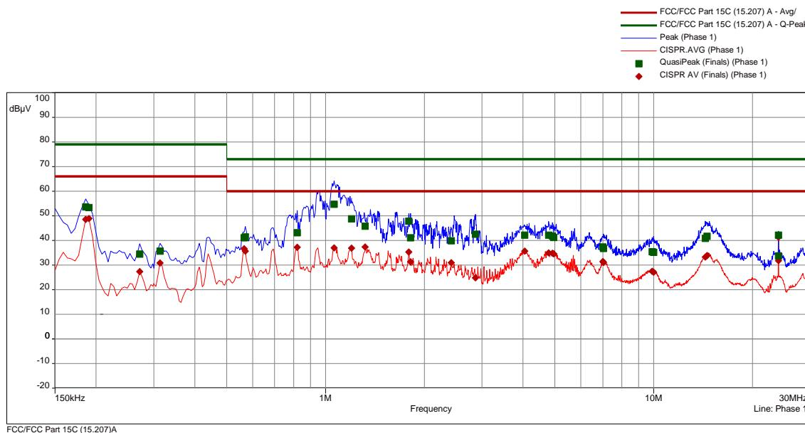
Phase 1, UWB and digital circuitry for UWB generation OFF
