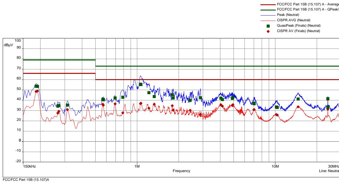
Note: There is no difference between the graphs. According to § 15.521(c), the emissions are assessed under Subpart B, see test report 80119127-03 of test laboratory CSA Group Bayern GmbH.
