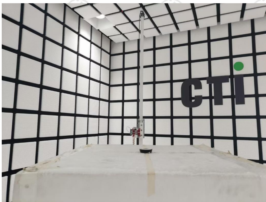
Radiated spurious emission Test Setup-2(Above 1GHz)
