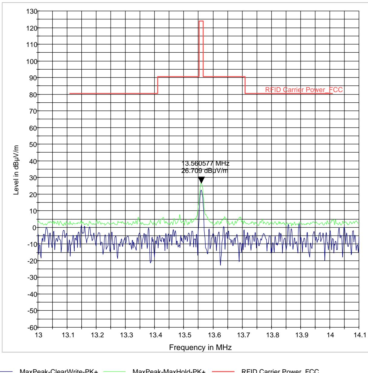
The red colored line shows the limit per part 15.225 extrapolated to 3m distance according to 15.31(f)(2), i.e. 40dB/decade.
