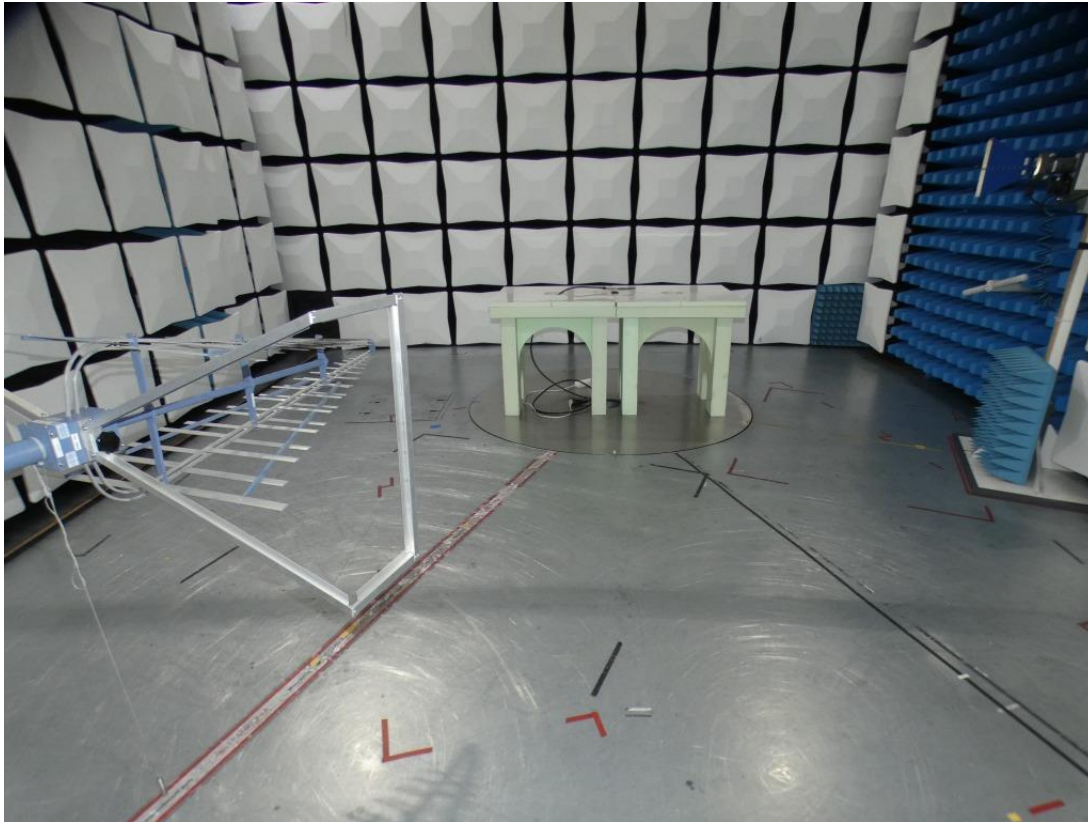
Photo 2: Test setup for radiated measurements (30 MHz - 1 GHz)
