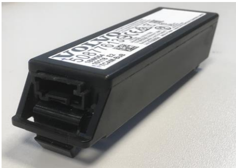
Figure: Backup Battery
