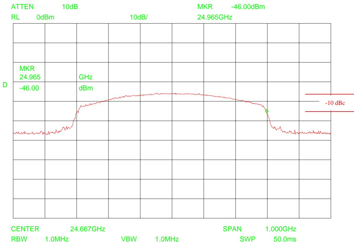
$$\text{High Frequency (F}_H\text{)} = 24.965 \text{ GHz (-10 dBc)}$$
