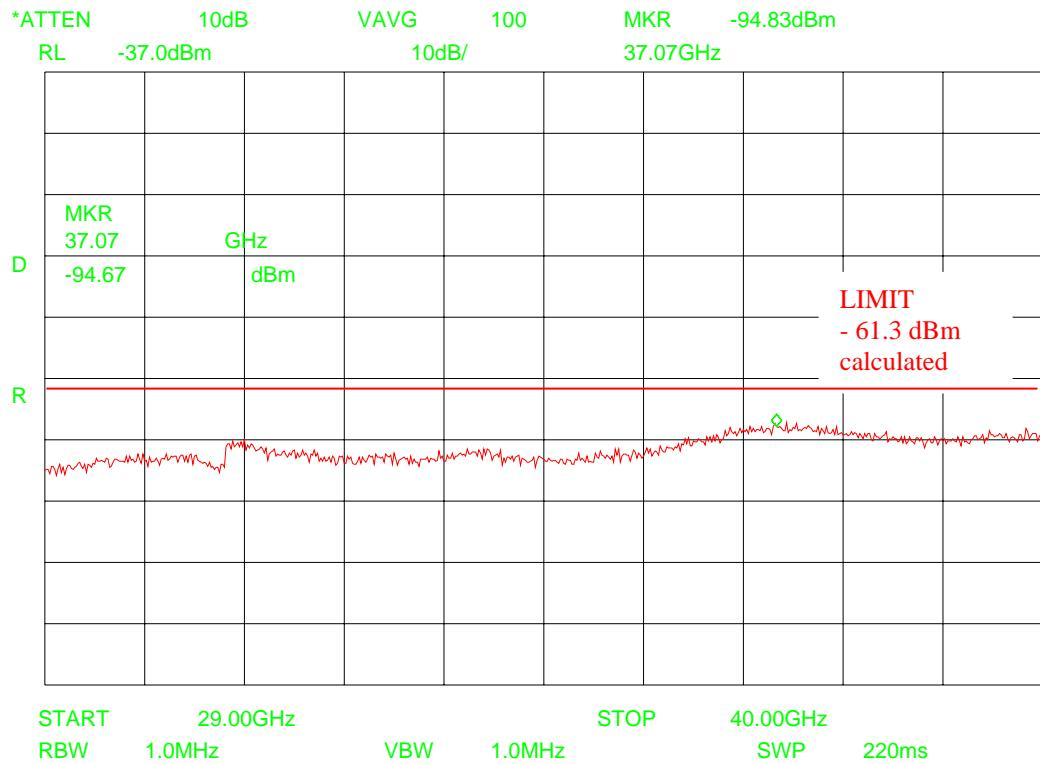
$P_{\text{Analyser}} = -94.6 \text{ dBm}$  (The  $A_{\text{Freespacing}}$  and the  $A_{\text{Gain}}$  is calculated in the analyser reading)
