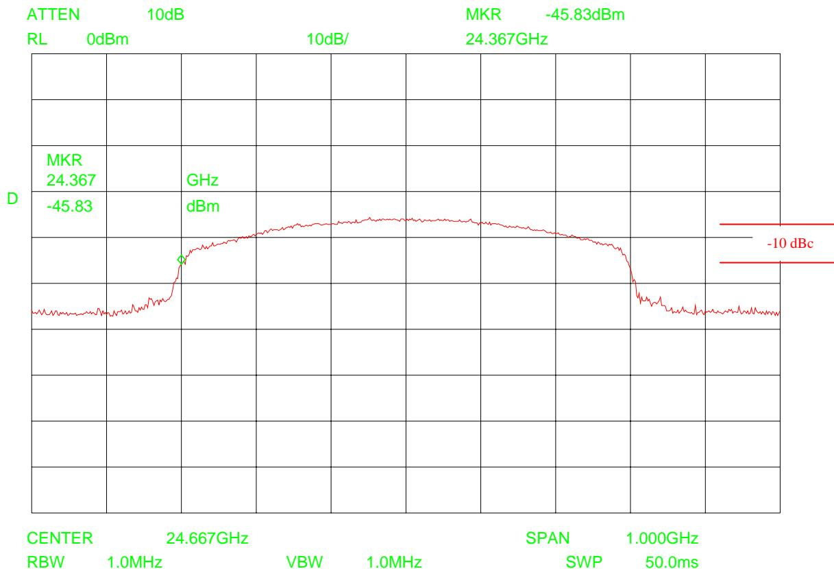
$$\text{Low Frequency (F}_L\text{)} = 24.367 \text{ GHz (-10 dBc)}$$
