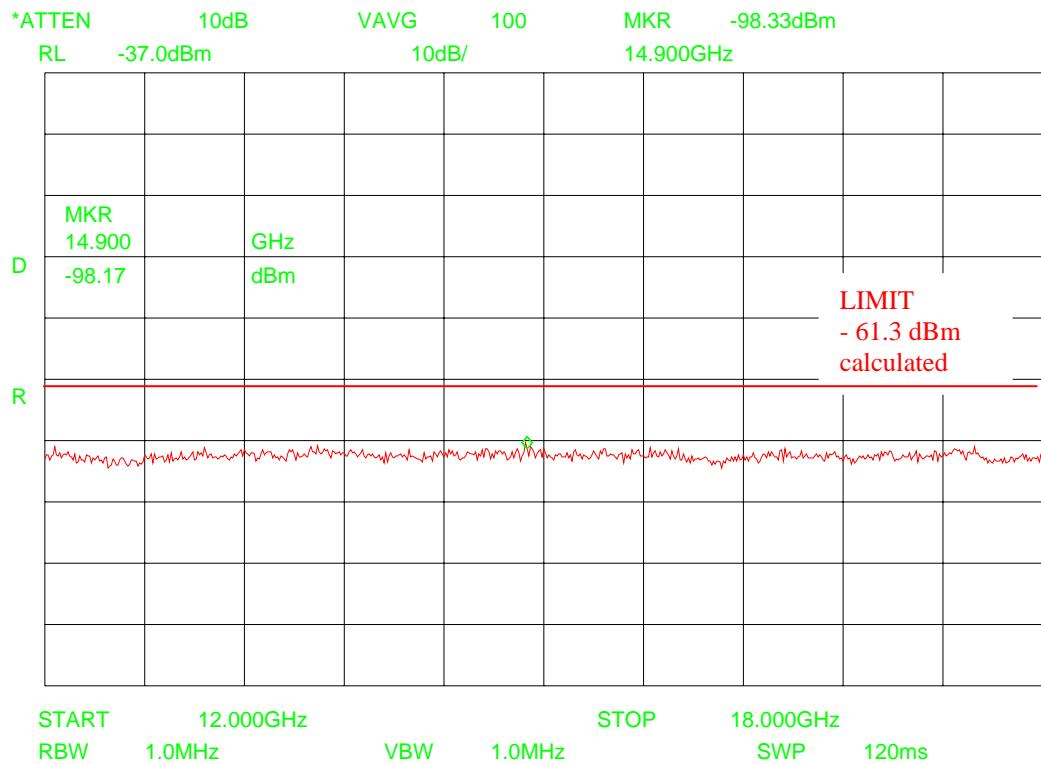
$P_{\text{Analyser}}$  = - 98.1 dBm (The  $A_{\text{Freespacing}}$  and the  $A_{\text{Gain}}$  is calculated in the analyser reading)
