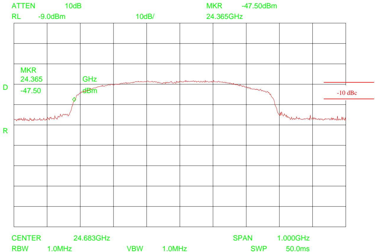
$$\text{Low Frequency (F}_L\text{)} = 24.365 \text{ GHz (-10 dBc)}$$
