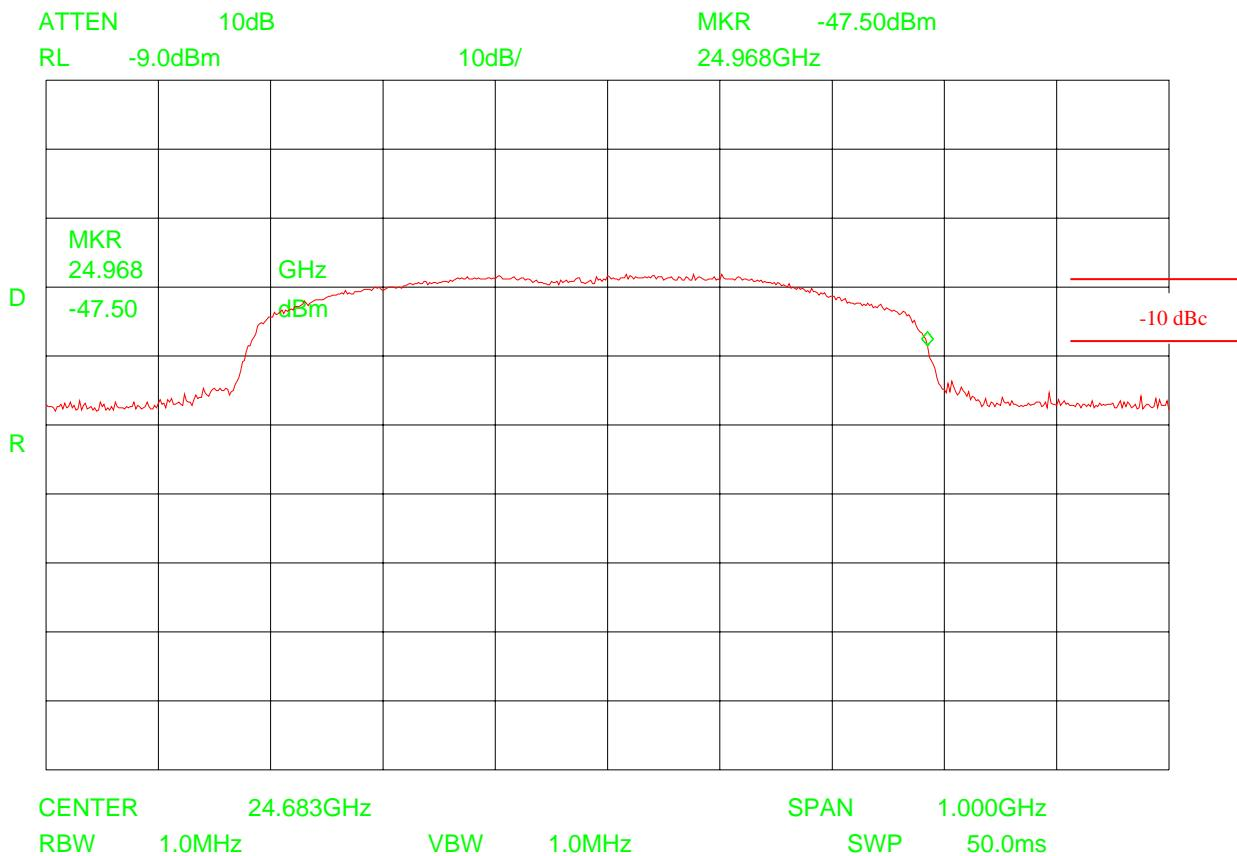
$$\text{High Frequency (F}_H\text{)} = 24.968 \text{ GHz (-10 dBc)}$$
