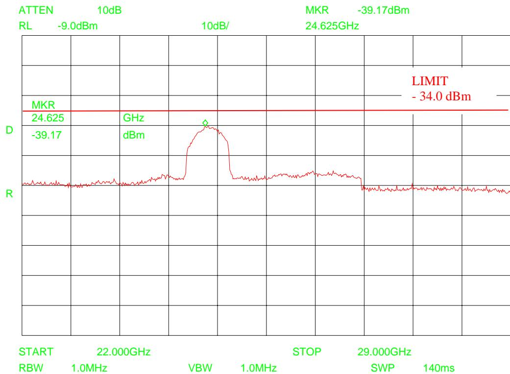
**This is a peak measurement with 1 MHz RBW/VBW according to FCC15.252 (b)(4)**
