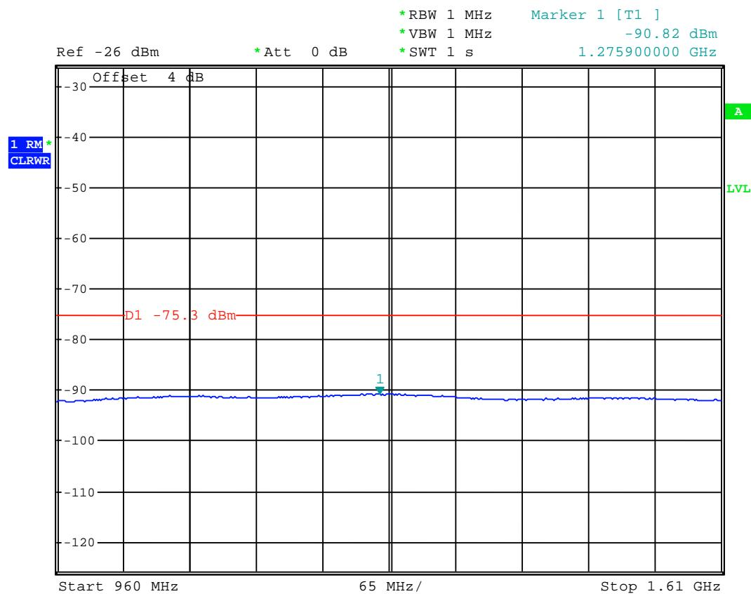
$P_{\text{Analyser}}$  = -90.8 dBm (The  $A_{\text{Freespacing}}$ , the  $A_{\text{Gain}}$  and  $P_{\text{Cable}}$  and Amplifier is calculated in the analyser reading)
