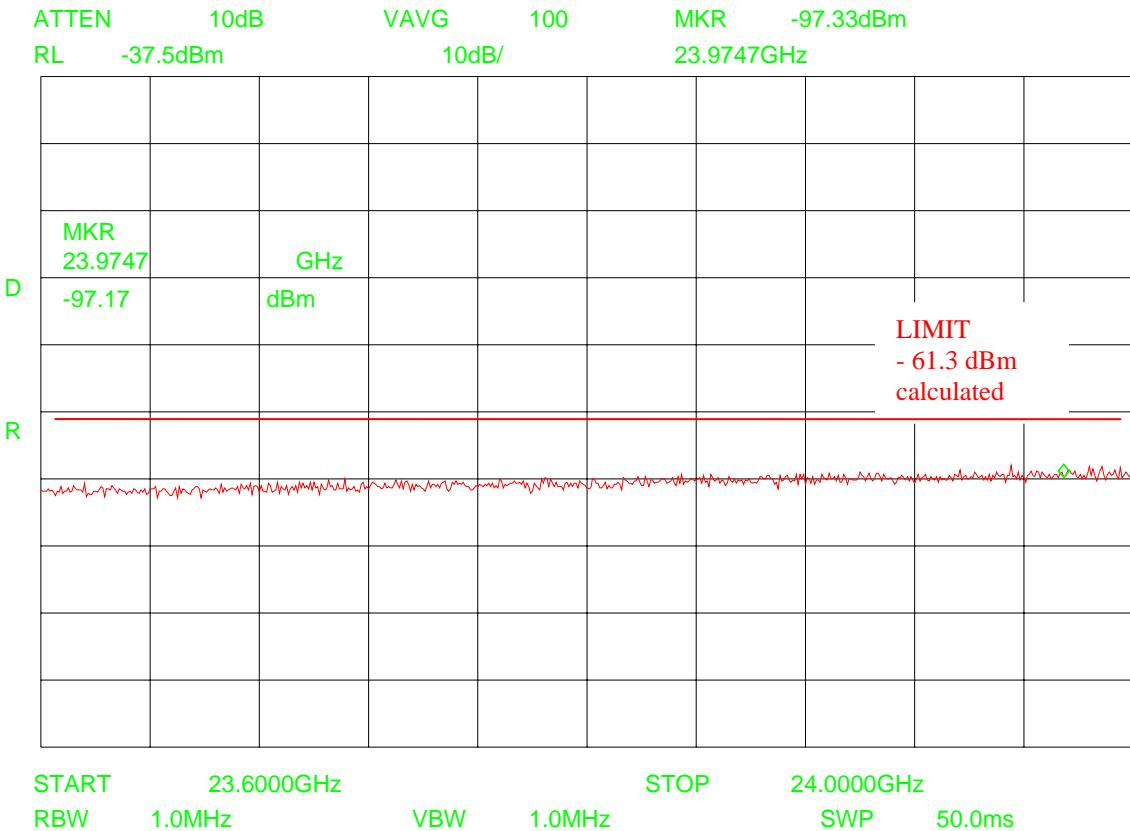
$P_{\text{Analyser}} = -97.1 \text{ dBm}$  (The  $A_{\text{Freespacing}}$  and the  $A_{\text{Gain}}$  is calculated in the analyser reading)
