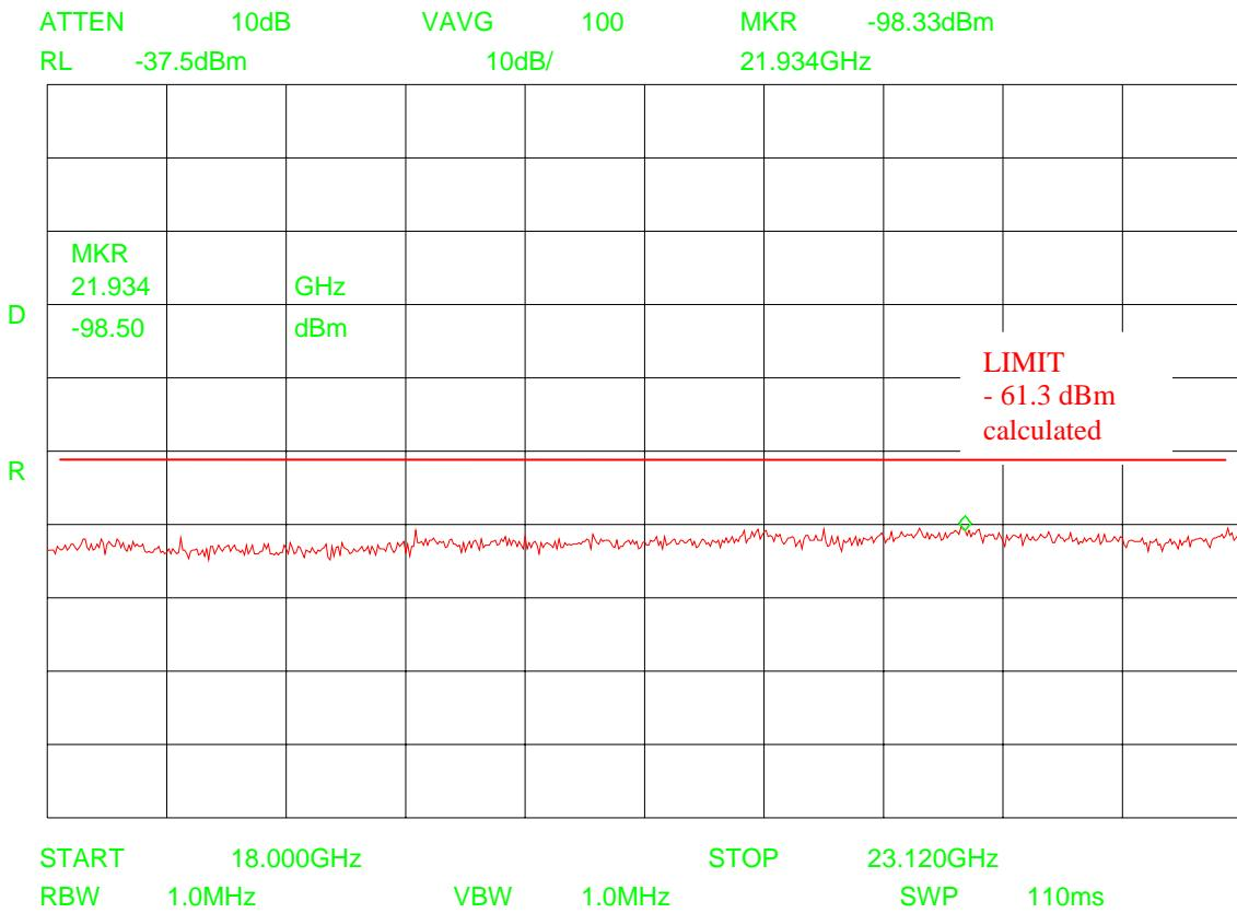
$P_{\text{Analyser}}$  = - 98.5 dBm (The  $A_{\text{Freespacing}}$  and the  $A_{\text{Gain}}$  is calculated in the analyser reading)
