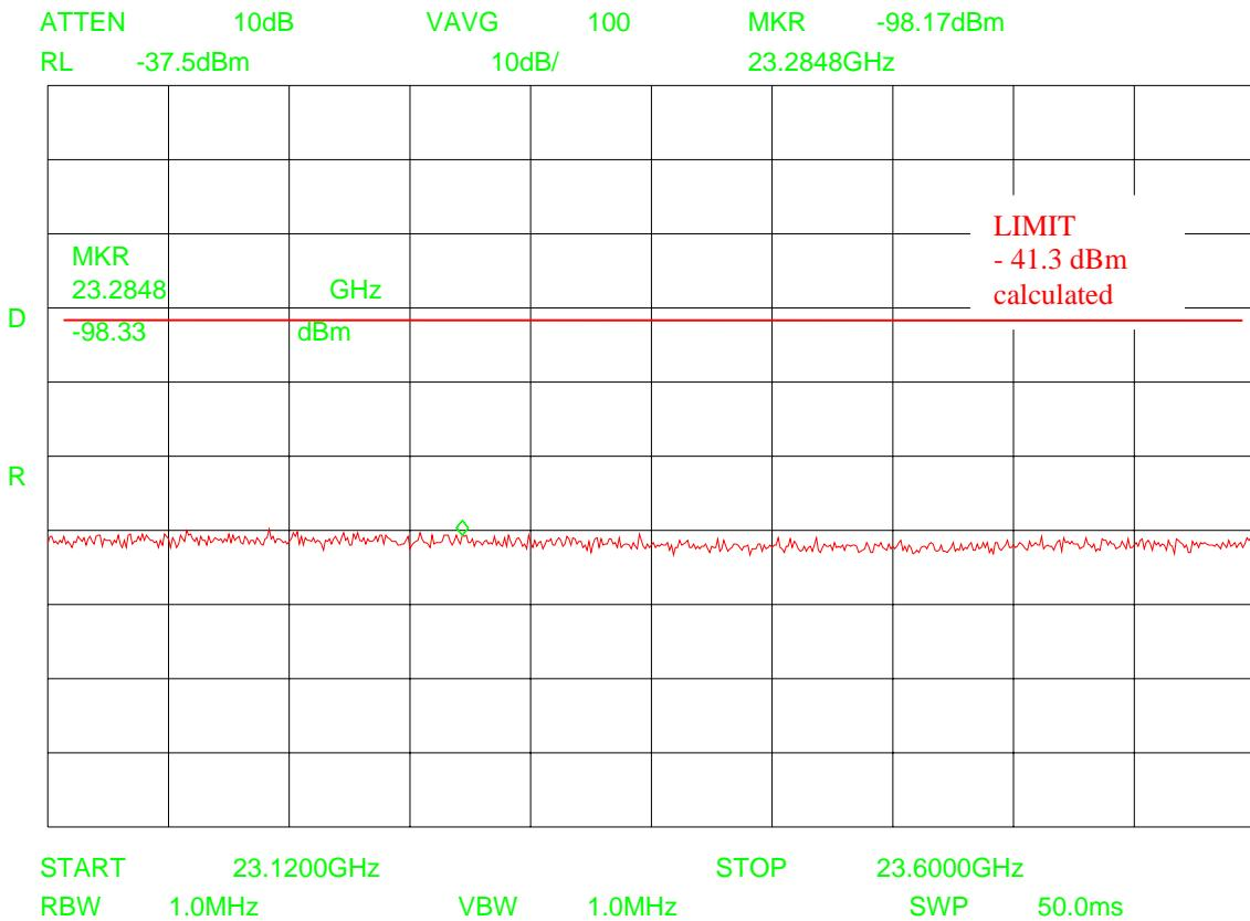
$P_{\text{Analyser}}$  = - 98.3 dBm (The  $A_{\text{Freespacing}}$  and the  $A_{\text{Gain}}$  is calculated in the analyser reading)
