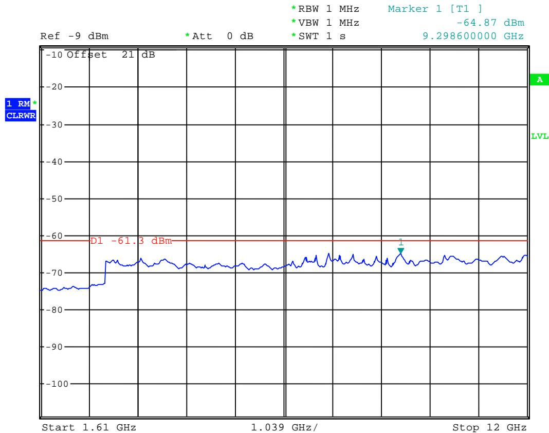
$P_{\text{Analyser}}$  = - 64.8 dBm (The  $A_{\text{Freespacing}}$ , the  $A_{\text{Gain}}$  and  $P_{\text{Cable}}$  and Amplifier is calculated in the analyser reading)
