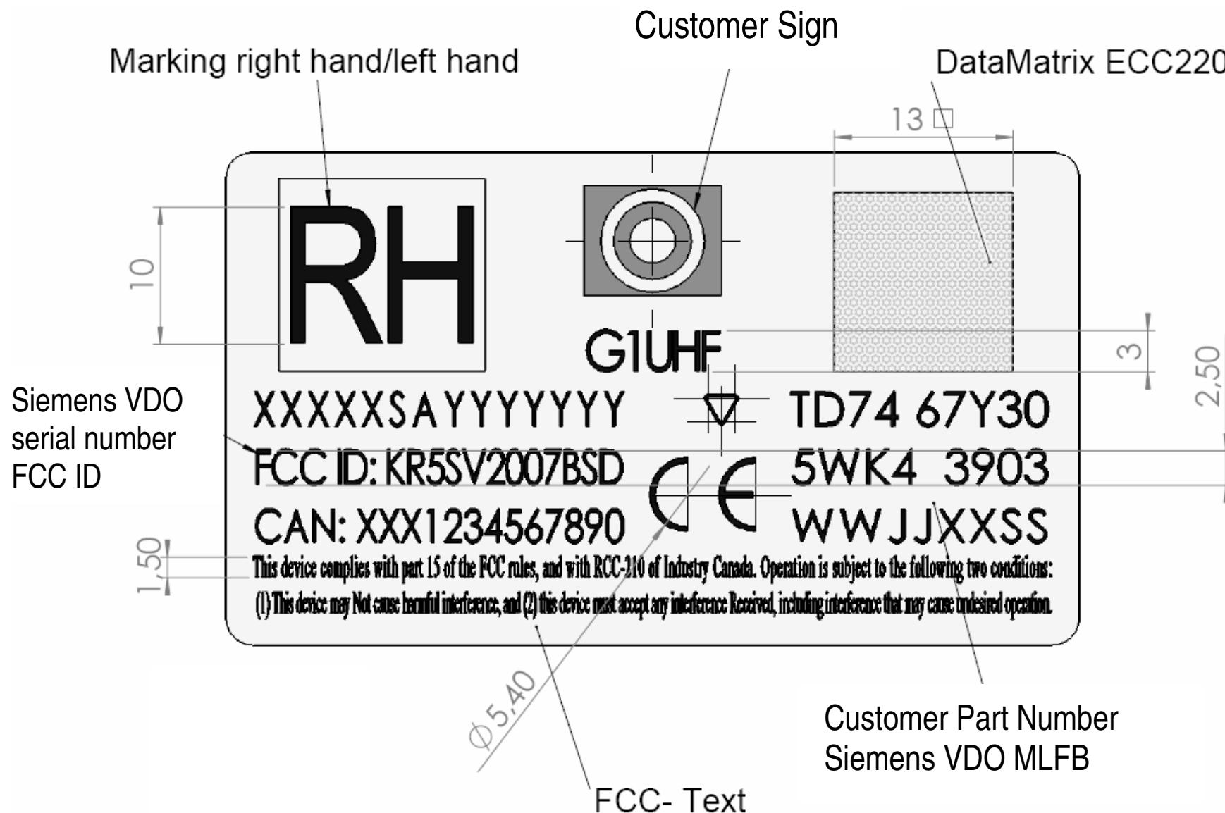
The product label is a permanent adhesive fixed on the rear sensor housing as shown in the above drawing. The label is designed to last the expected lifetime of the radar device in the environment in which the equipment is operated and is not readily detachable.
