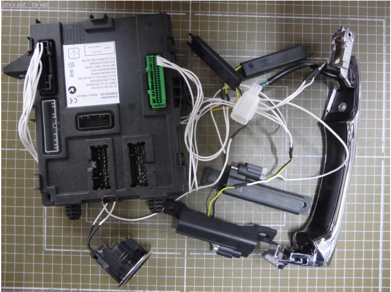
LF system antenna configuration
