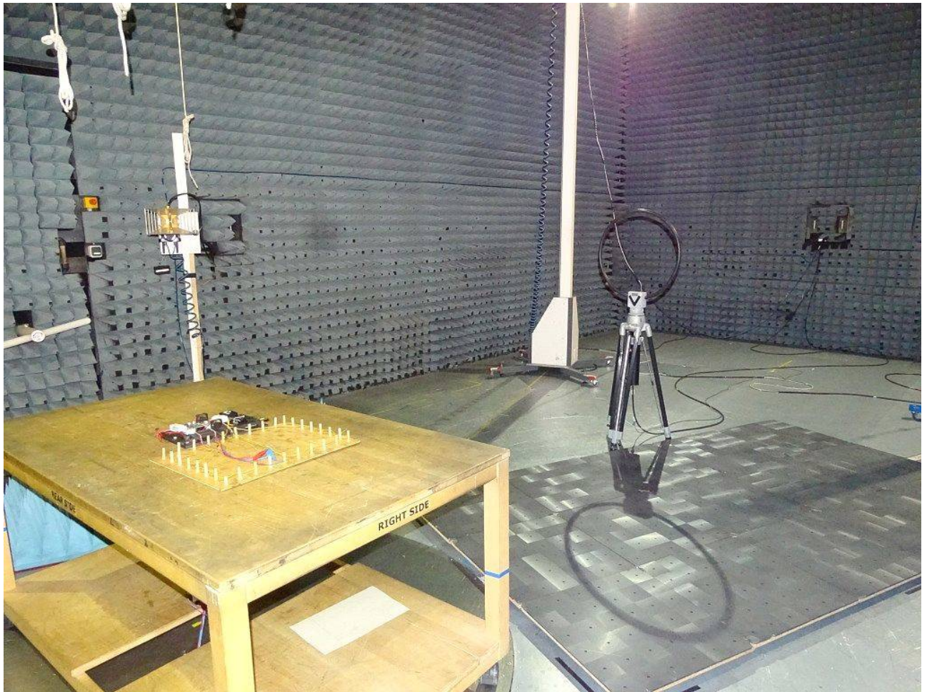
Photo 1: Test setup for radiated measurements (Enclosure, semi-anechoic chamber, 9 kHz to 30 MHz, intentional radiator §15, ANSI C63.10)
