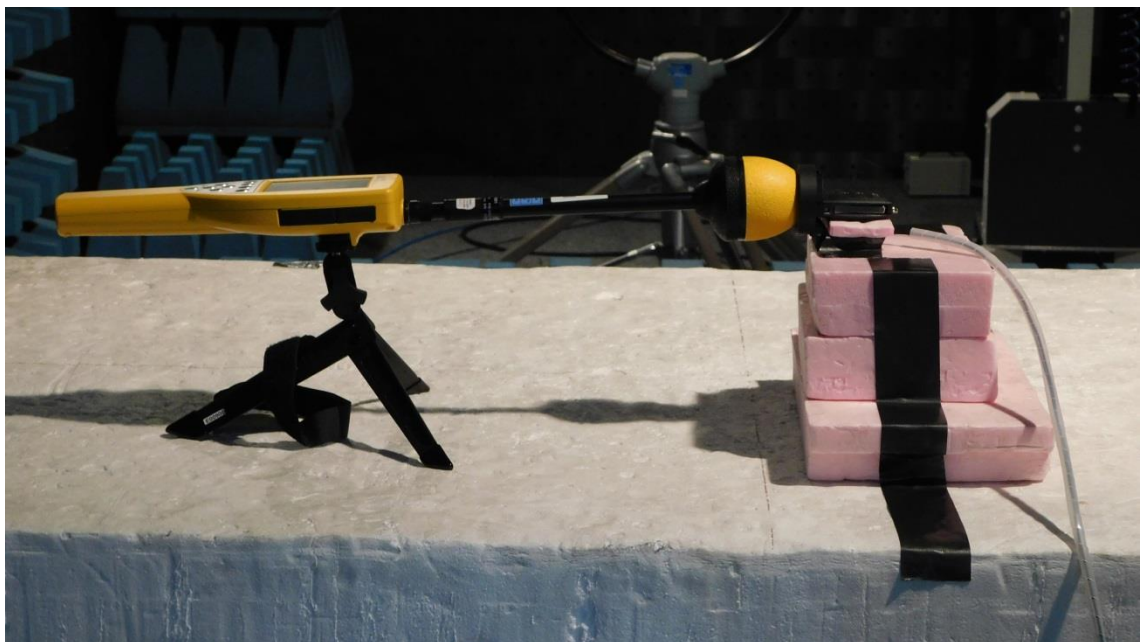
Picture 4: Setup of electric field test at a measurement distance of 0 cm, mode 2
