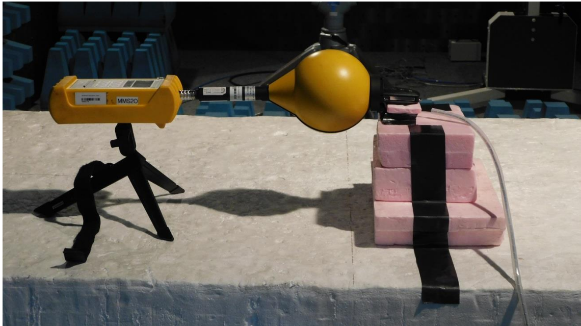
Picture 3: Setup of magnetic field test at a measurement distance of 0 cm
