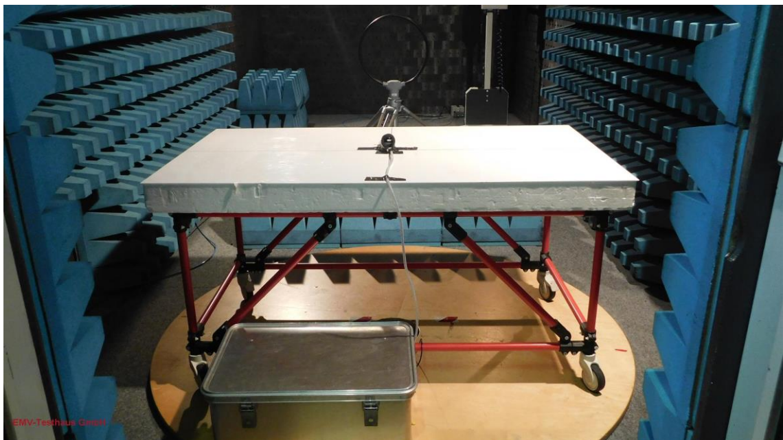
Picture 2: EUT test setup radiated emission test 9 kHz – 30 MHz (rear view)
