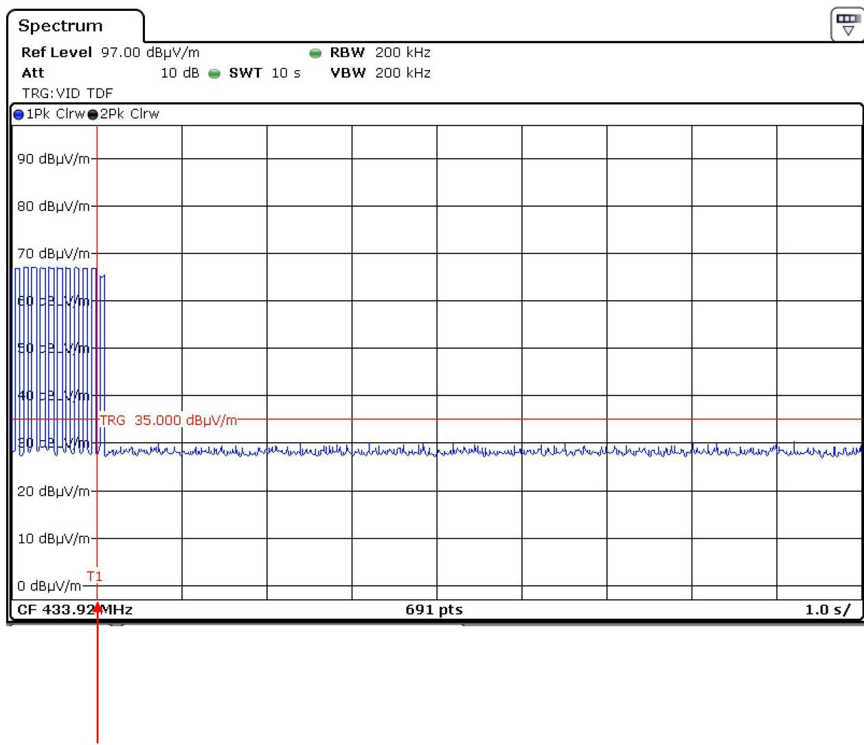
The transmission times are for all buttons nearly the same! The worst case transmission times was recorded!
