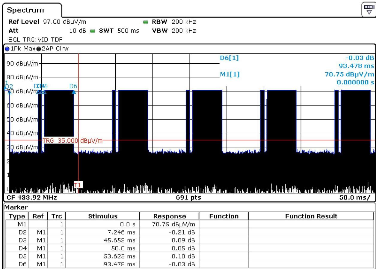
**The transmission times are for all buttons nearly the same! The worst case transmission times was recorded!**
