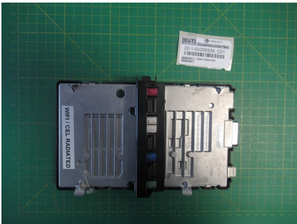
Fig. Ext.: 2 : Ext. - Rear Telematic Control Unit
