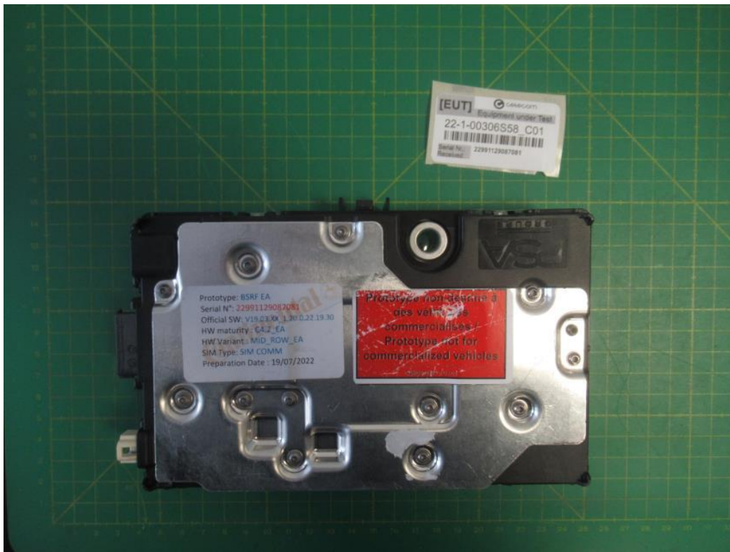
Fig. Ext.: 1 : Ext. - Front Telematic Control Unit
