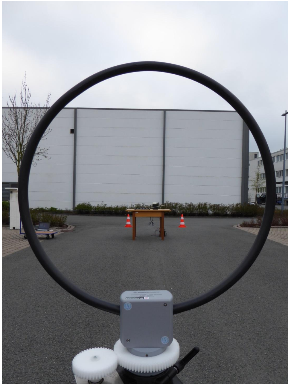
154295_23.JPG: Test setup outdoor test site (9 kHz to 30 MHz)
