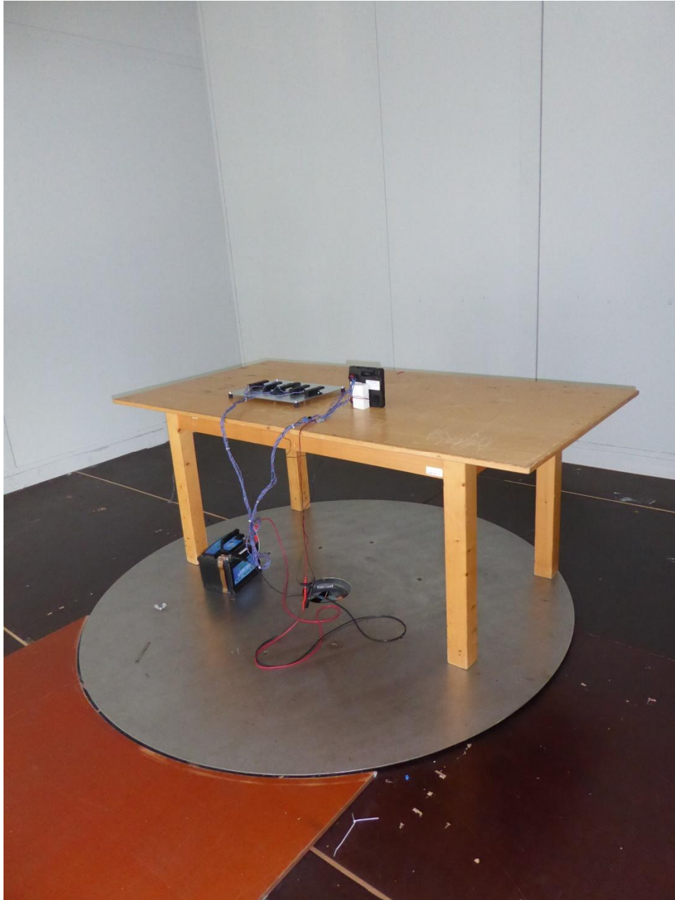
154295_24.JPG: Test setup open area test site (30 MHz to 1 GHz)
