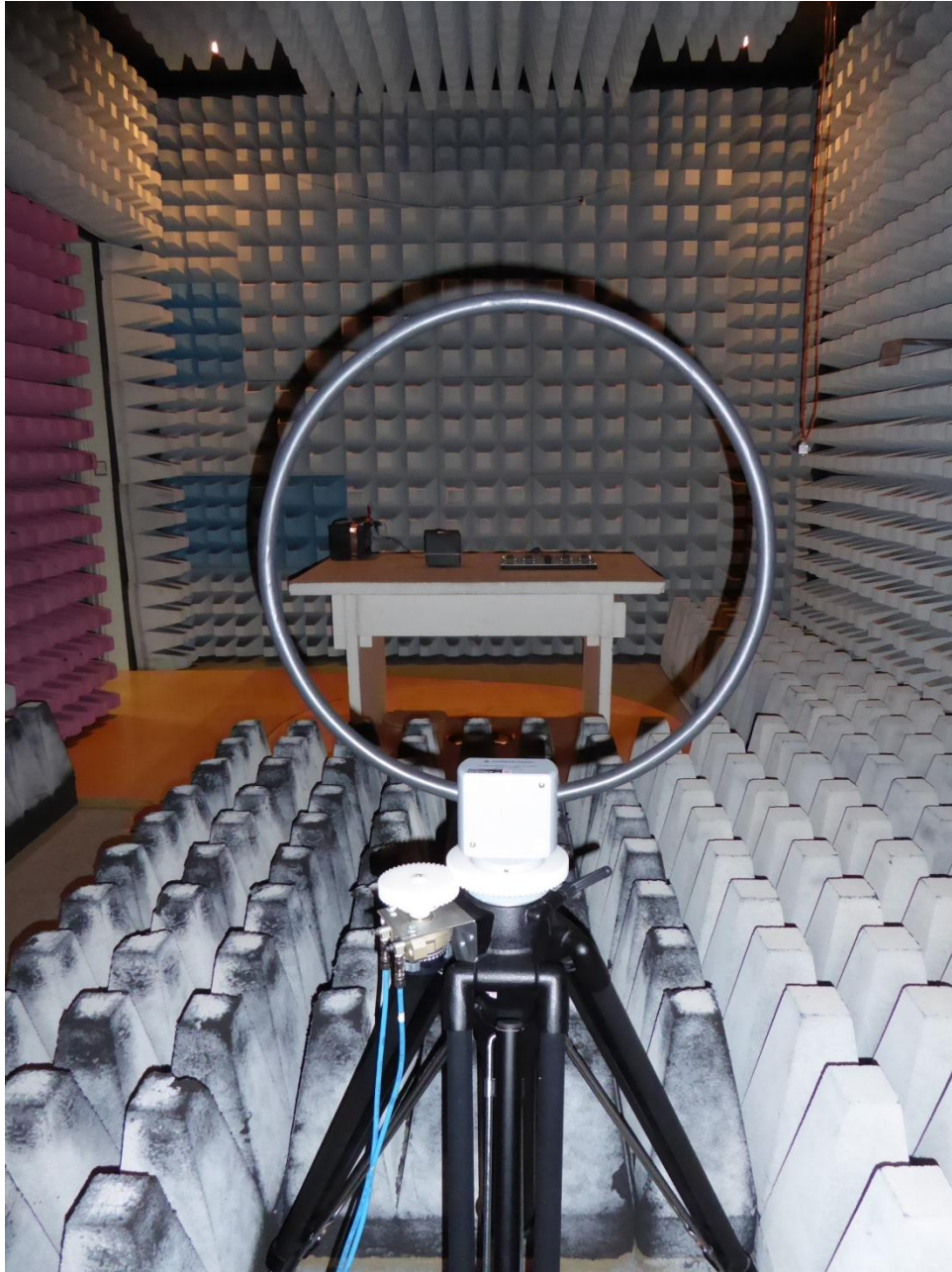
154295_20.JPG: Test setup fully anechoic chamber (9 kHz to 30 MHz)
