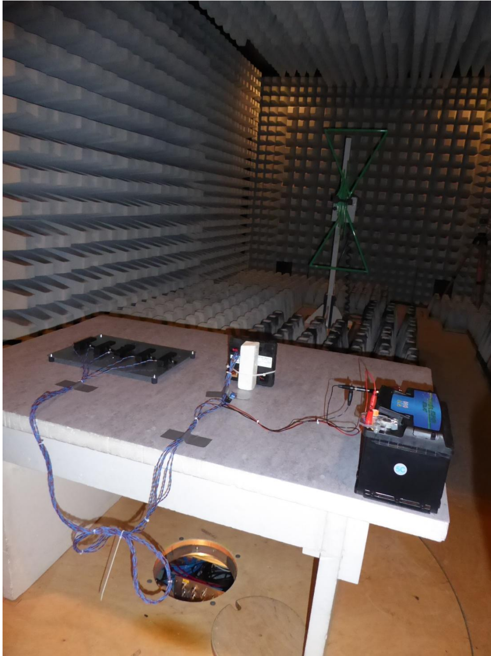
154295_20.JPG: Test setup fully anechoic chamber (30 MHz to 1 GHz)
