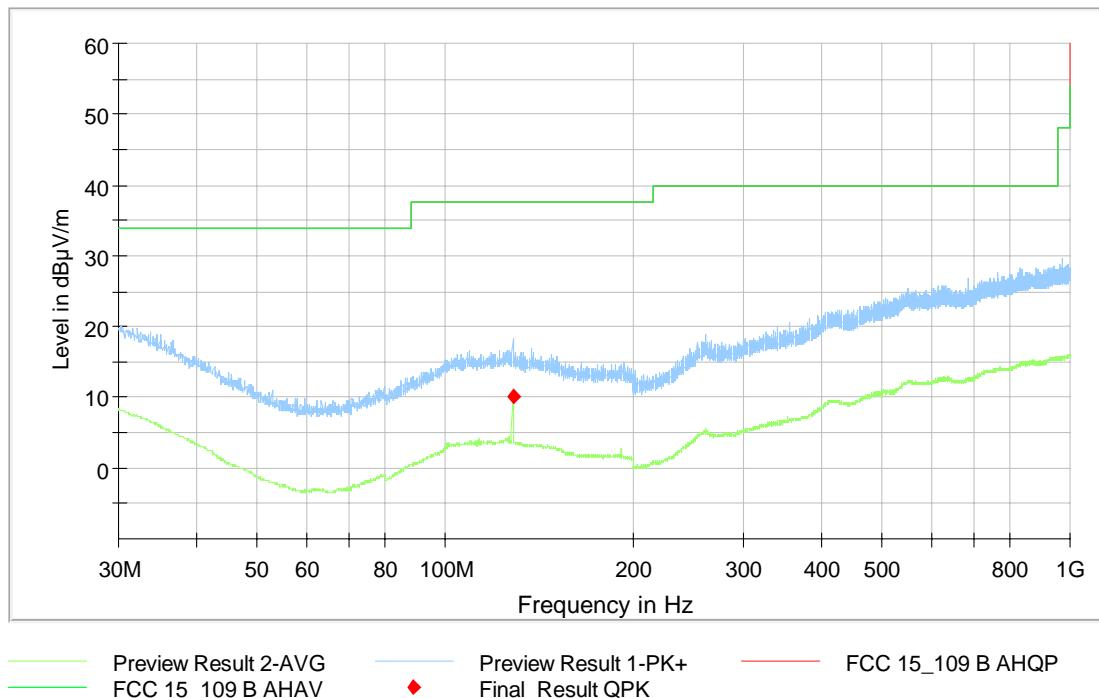
The following frequency was found inside restricted bands during the preliminary emission measurement from 30 MHz to 1 GHz: 128.052 MHz
