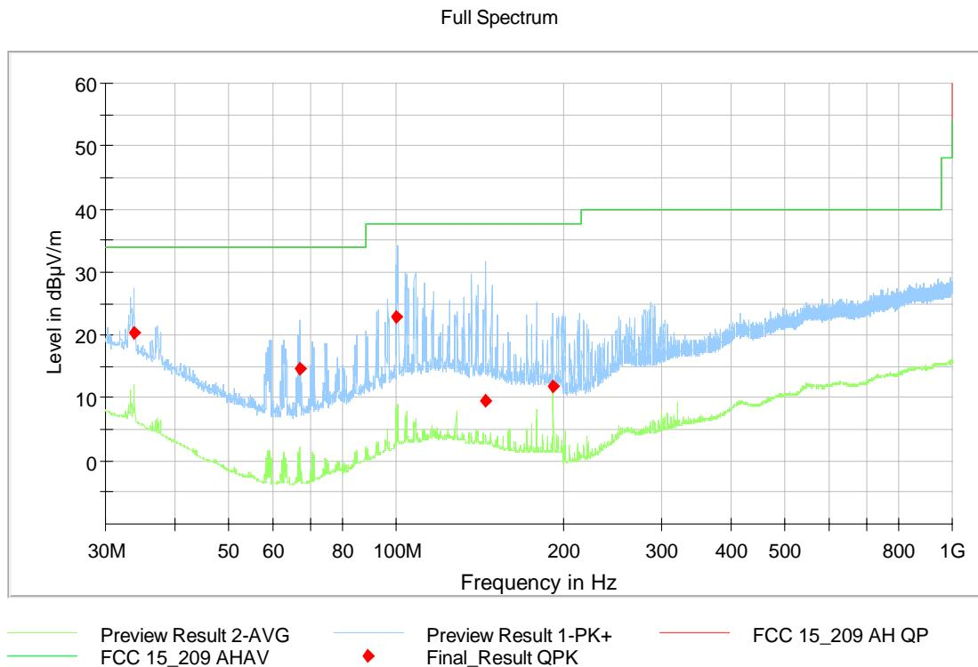
No frequencies were found inside the restricted bands during the preliminary radiated emission test.
