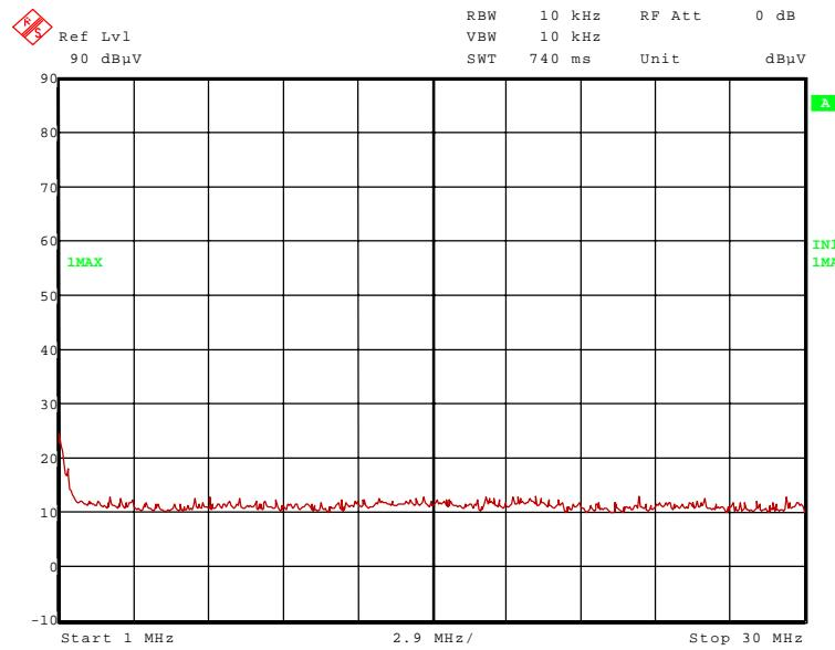
The following frequencies were found inside restricted bands during the preliminary emission measurement from 9 kHz to 30 MHz:
