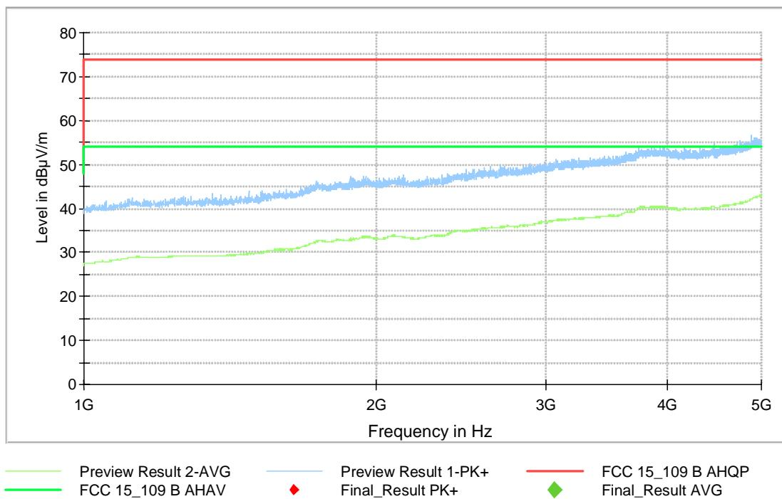
No significant emission was found. The maximum peak noise level was measured at 4.876 GHz with a level of 56.5 dB $\mu$ V/m results to a margin of 17.5 dB to the limit. The maximum average noise level was measured at 5.0 GHz with a level of 42.9 dB $\mu$ V/m results to a margin of 11.1 dB.
