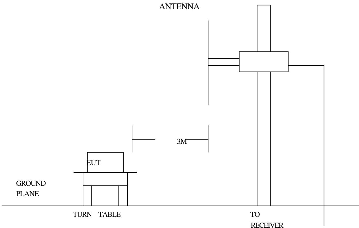
**5 . 3 RADIATED TEST SET-UP**
