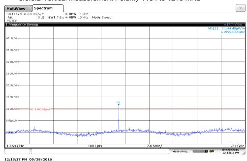
Note: Narrow band emission @ 1.19995 GHz fails under 15.209 limit
