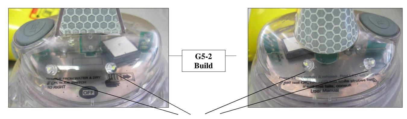
Four LEDs replace the single LED with lens for the Low-Duty-Cycle-Light function
