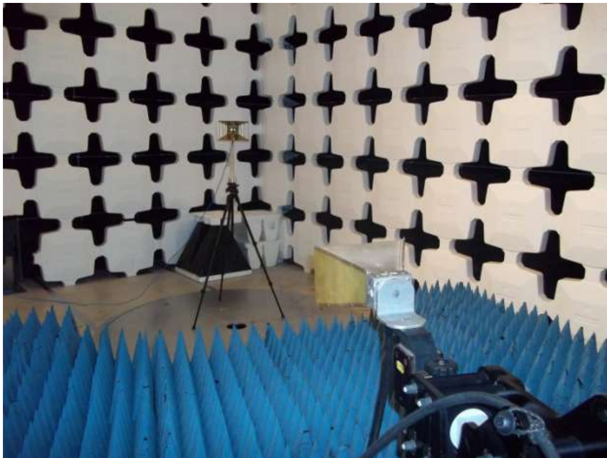
Figure 12. Substitution Testing above 1 GHz
