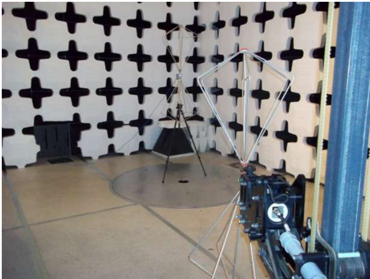
Figure 10. Substitution Testing 30-200 MHz
