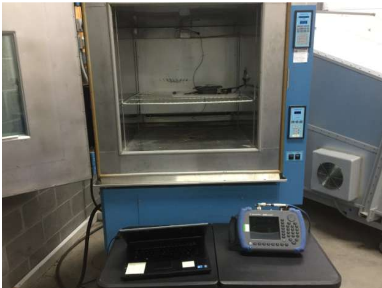
Figure 8. Frequency Stability Test Setup
