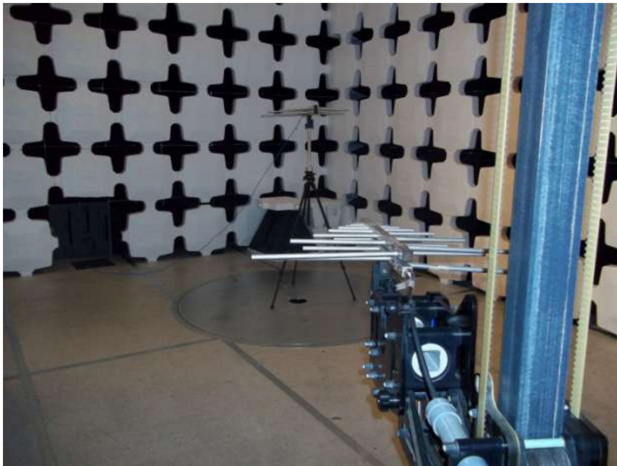
Figure 11. Substitution Testing 200 - 1000 MHz
