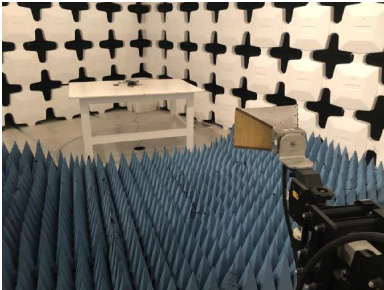
Figure 6. Radiated Emissions Test Setup, Above 1 GHz (Radio Test with EUT in worst case position)
