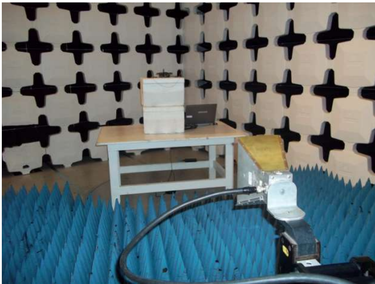
Figure 7. EUT above 1 GHz Test Configuration (Intentional Emissions)
