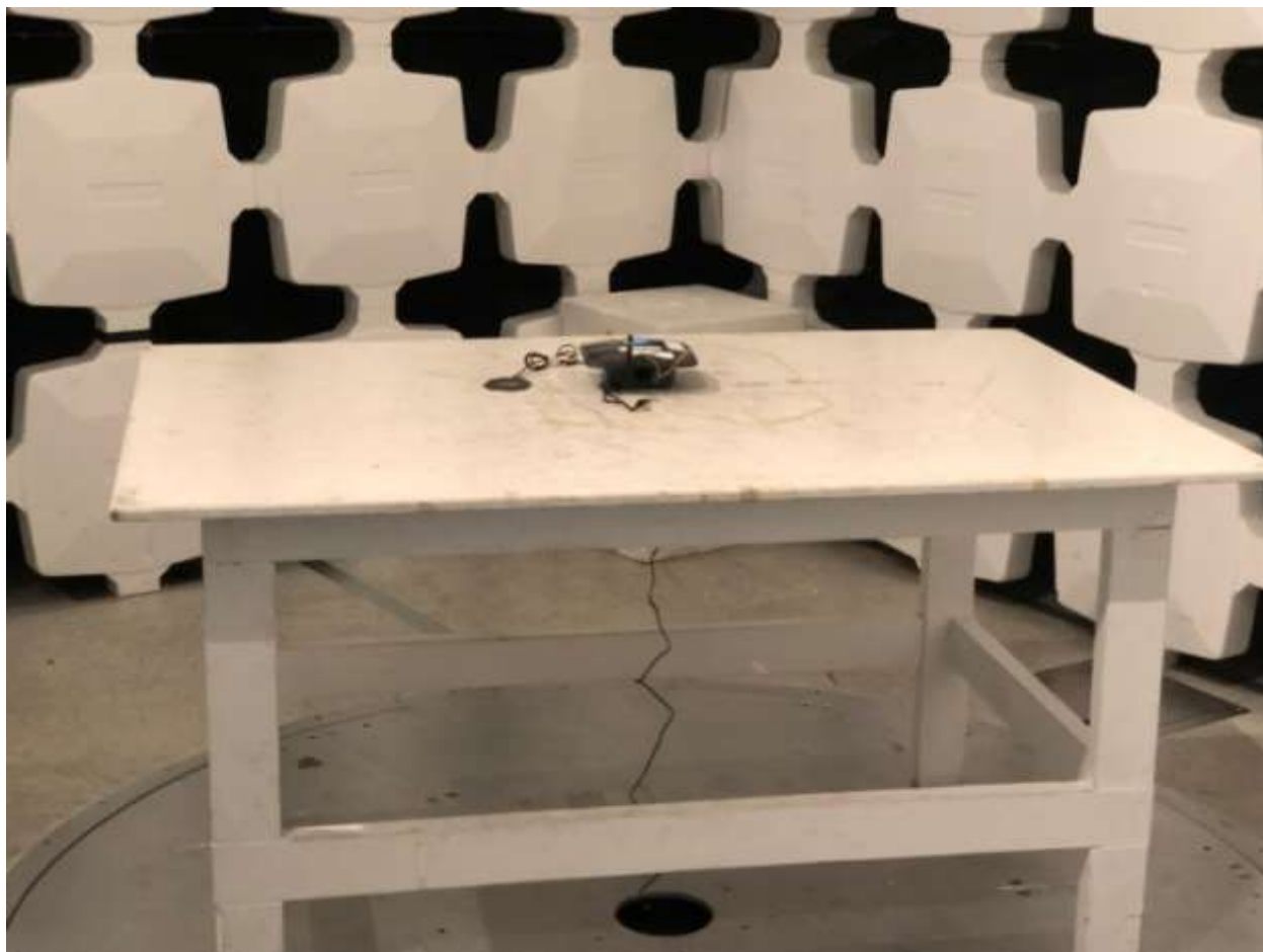
Figure 1. Radiated Emissions Test Setup, Close-Up
