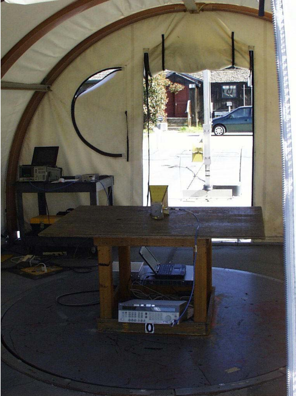
Substitution test set-up, 1-18 GHz
