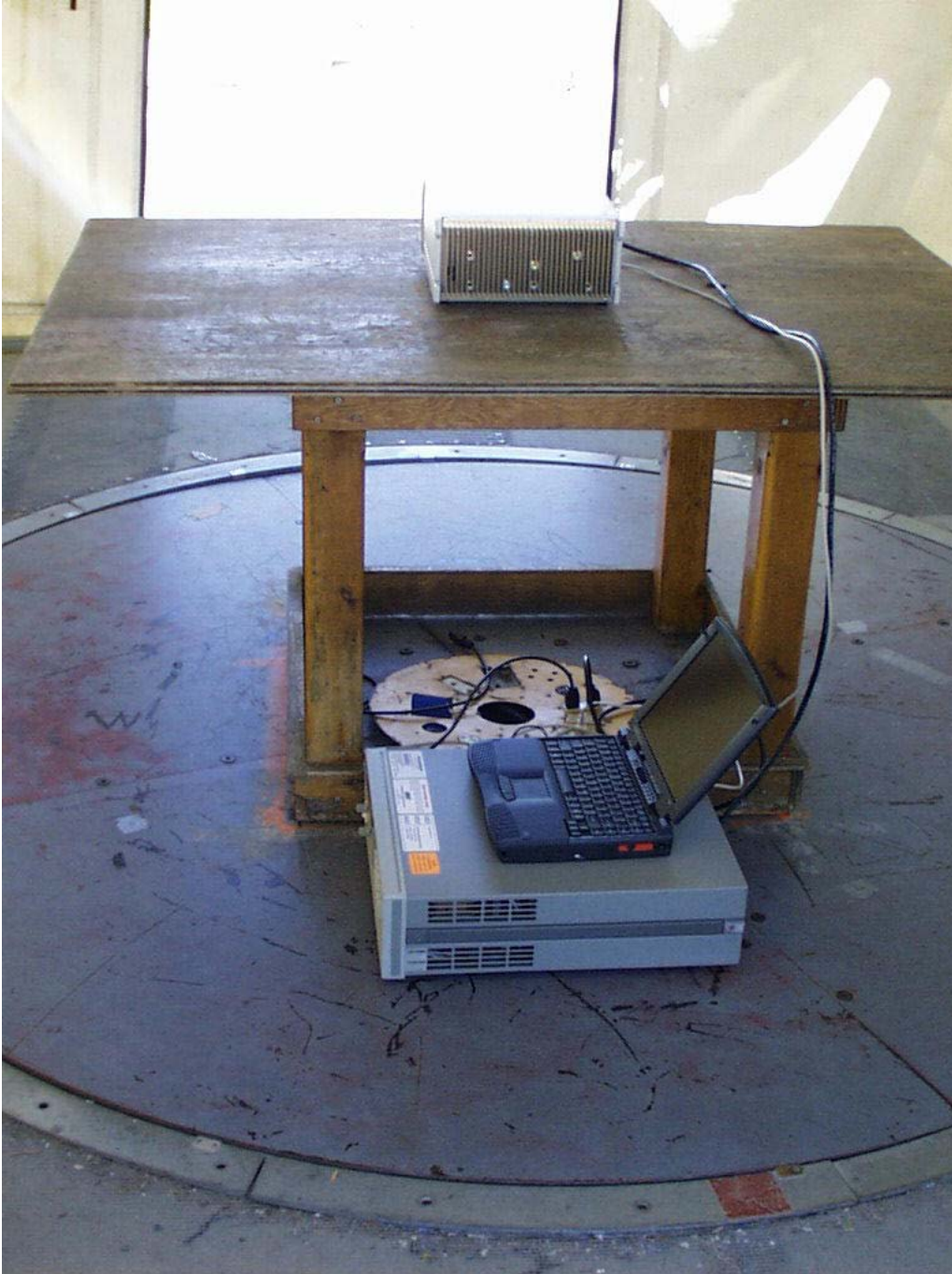
Radiated emissions, substitution method, equipment rear view
