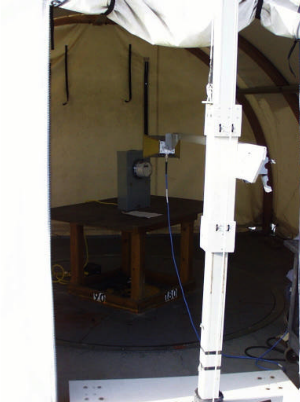
Radiated emissions test set-up
