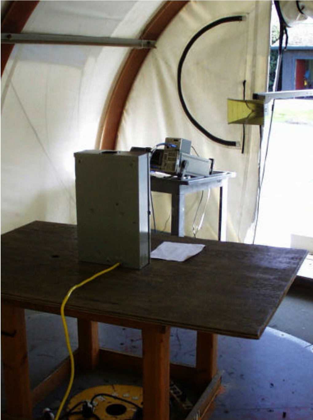
Radiated emissions test set-up
