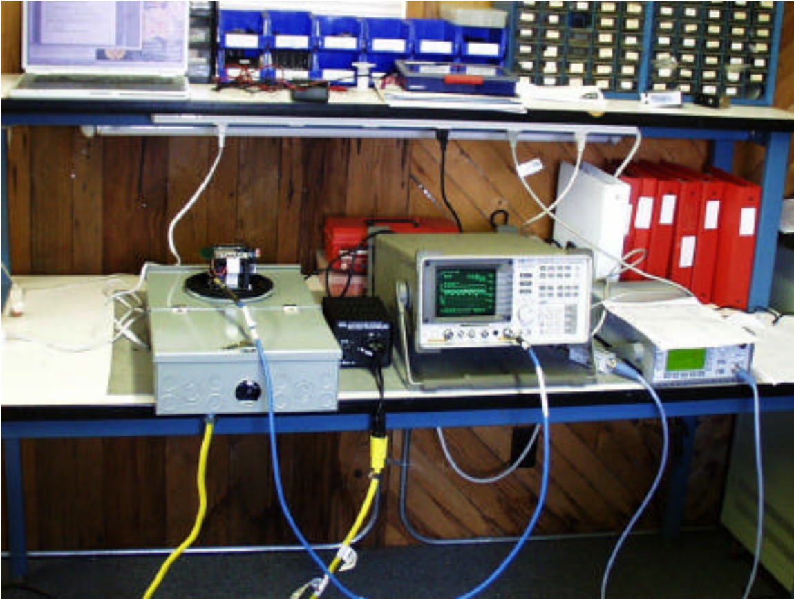
Antenna output conducted set-up
