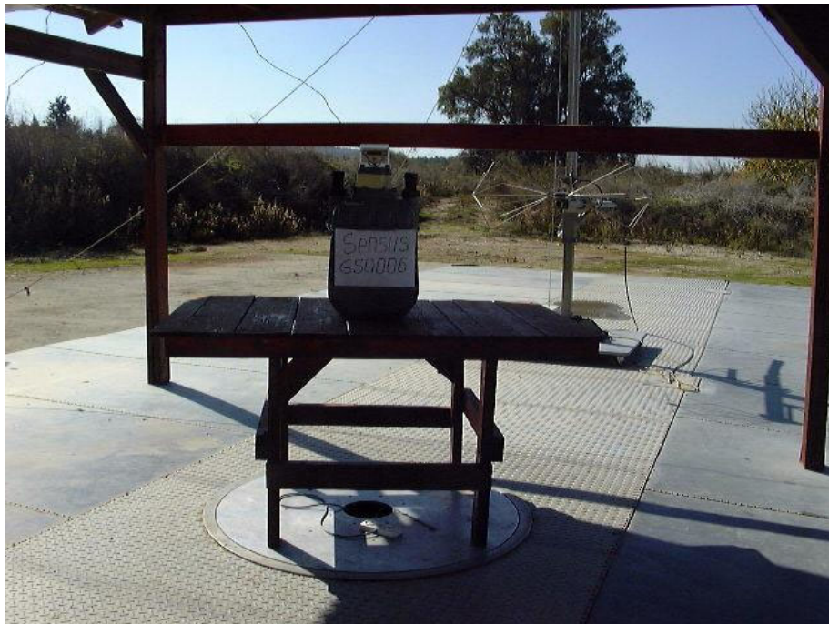
Figure 4. Spurious Radiated Emission Test Front
