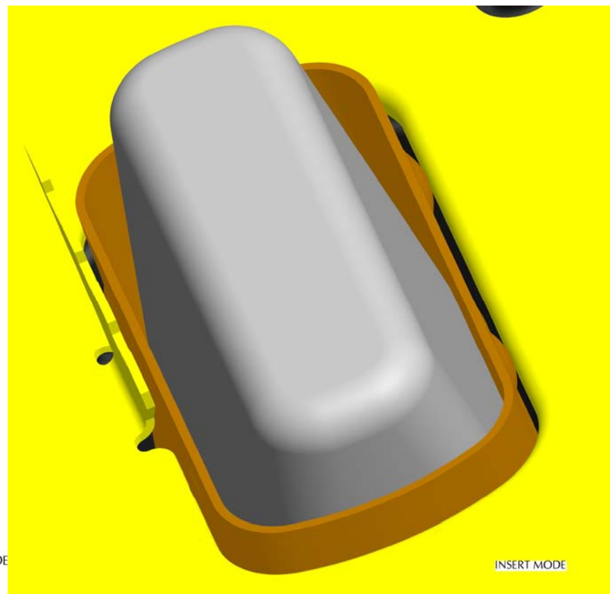
Figure 8 Mechanical Connection Between the Antenna Ground Plane and Transmitter Isolation Sleeve
