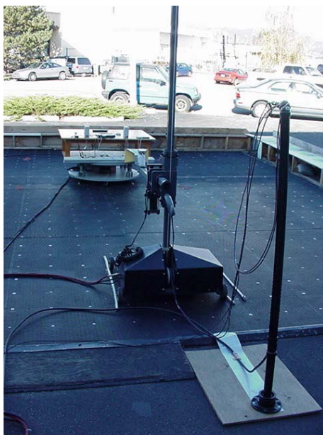
Photograph J.7-3 - Portable 3 m Horn setup
