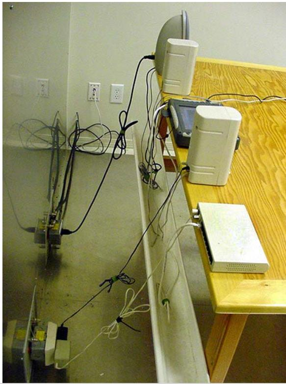
Photograph I-2 - AC Powerline Conducted Emission Configuration
