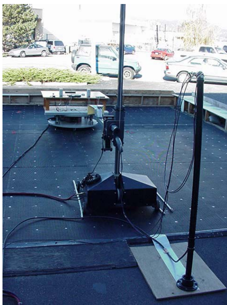
Photograph J.7-3 - Portable 3 m Horn setup
