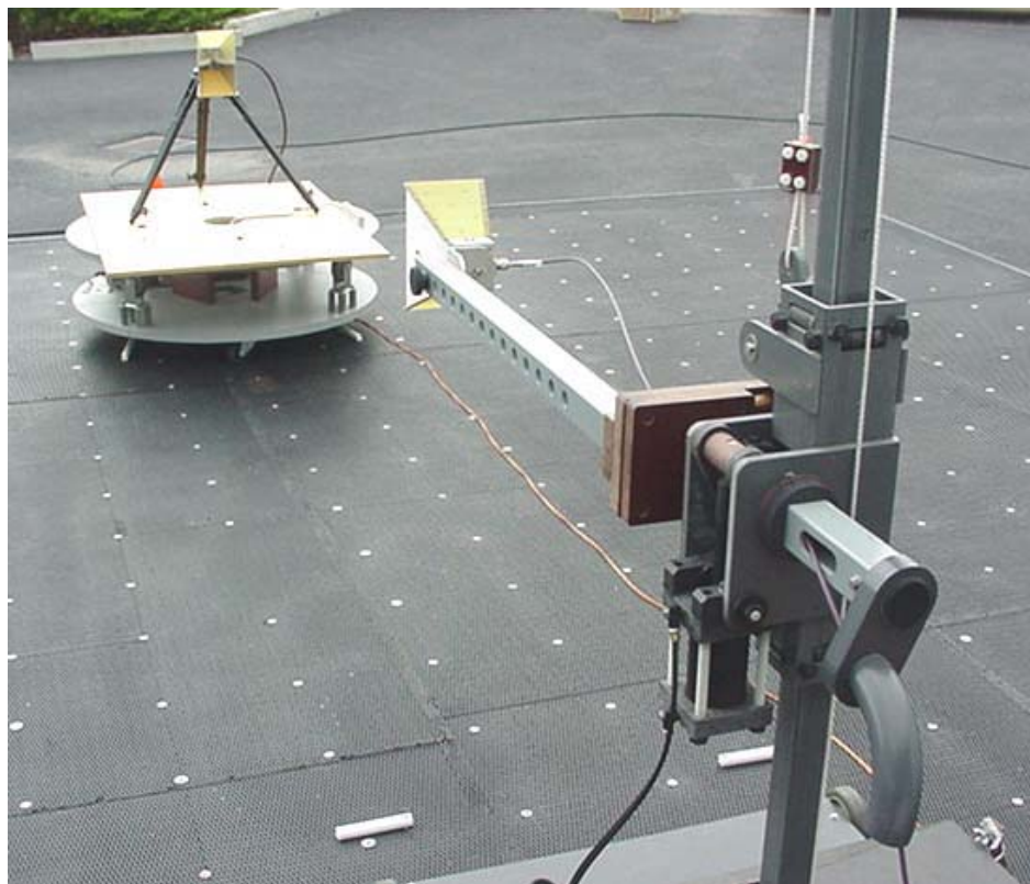
Substitution Horn antenna and Horn receive antenna
