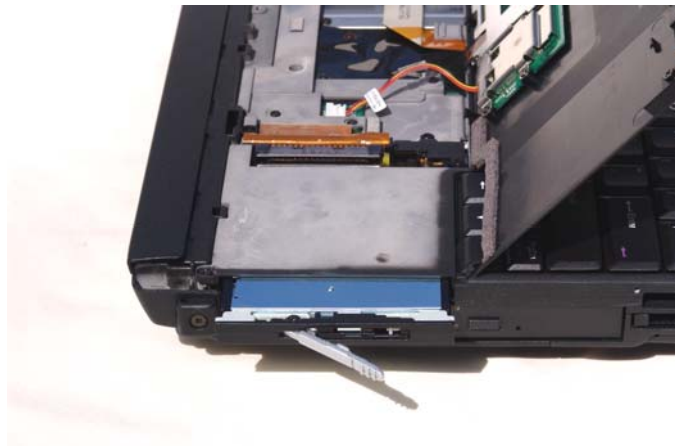
CRMA module with IX-MC5725 partially removed
