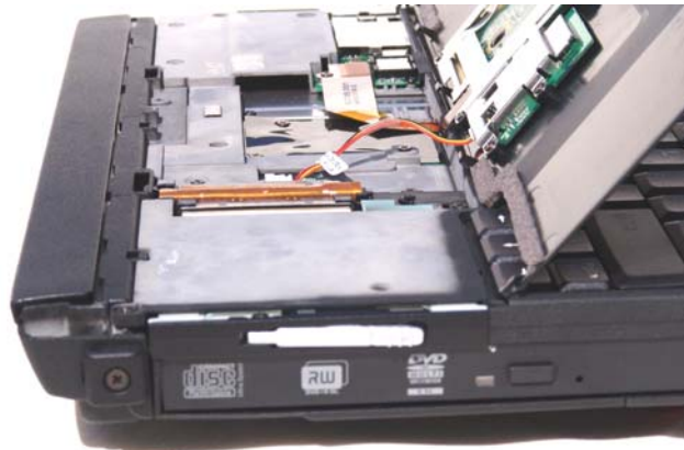
CRMA module with IX-MC5725 partially removed
