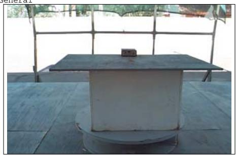
$\frac{\texttt{TEST SETUP}}{\texttt{g0060047:}} : \qquad \text{Radiated Emiss} \\ 2000-\texttt{Jun-14 Wed } 08:25:11$ Radiated Emissions
