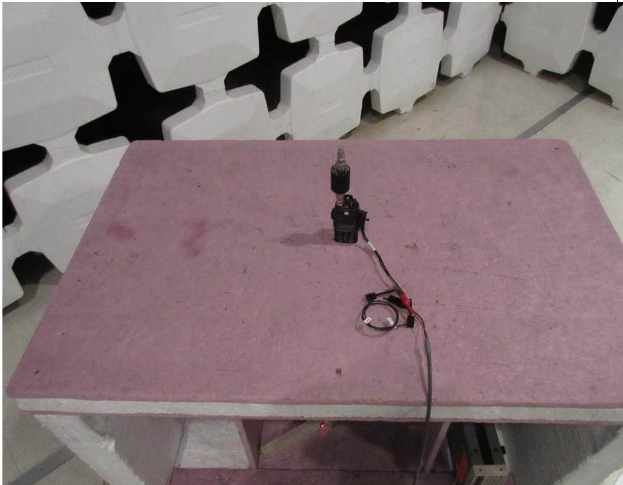
FIELD STRENGTH SPURIOUS EMISSIONS  $f < 30\text{MHz}$
