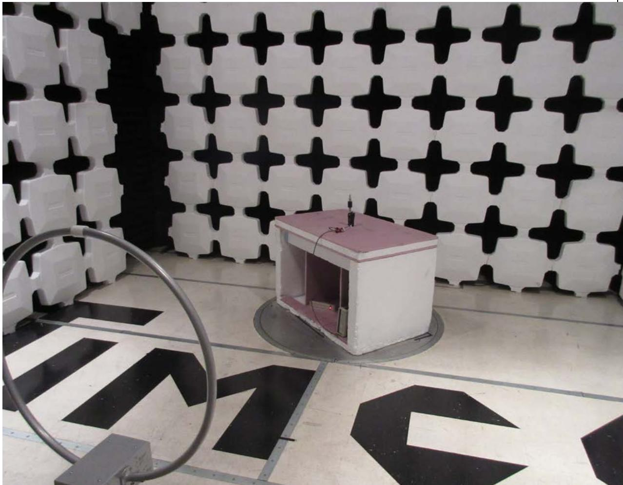
FIELD STRENGTH SPURIOUS EMISSIONS  $f < 200\text{MHz}$
