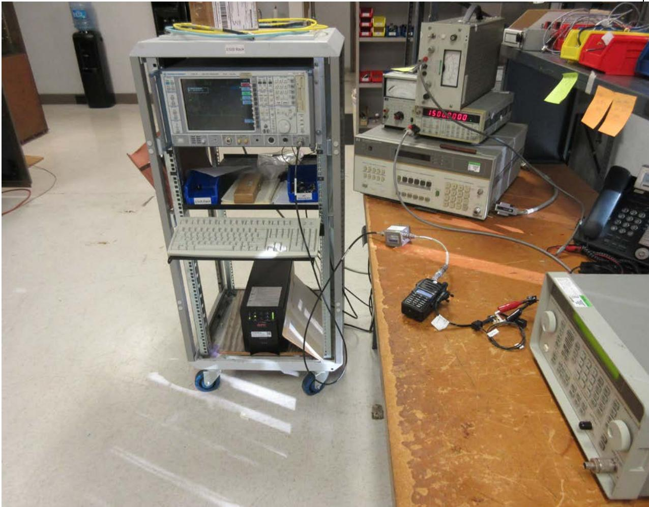
**FIELD STRENGTH SPURIOUS EMISSIONS TEST SETUP**
