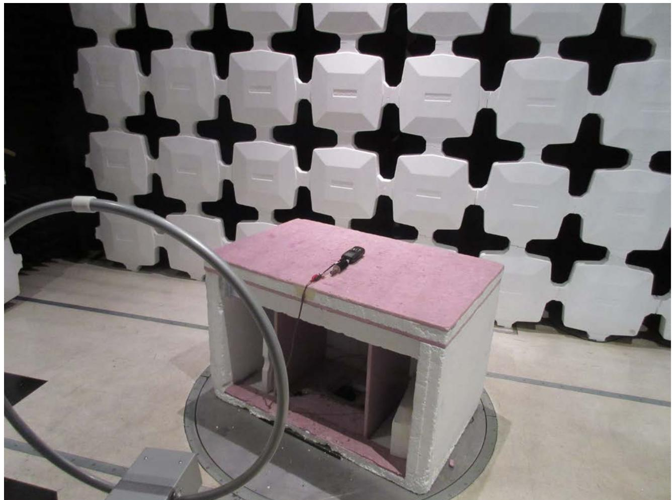
**FIELD STRENGTH SPURIOUS EMISSIONS – 30 MHz to 200 MHz**
