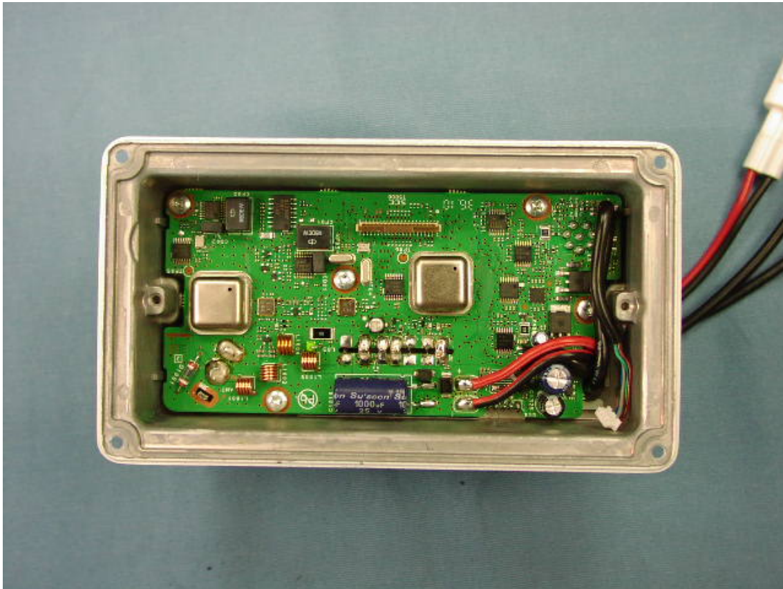
Chassis and Main-Unit (Removed Front-Panel)
