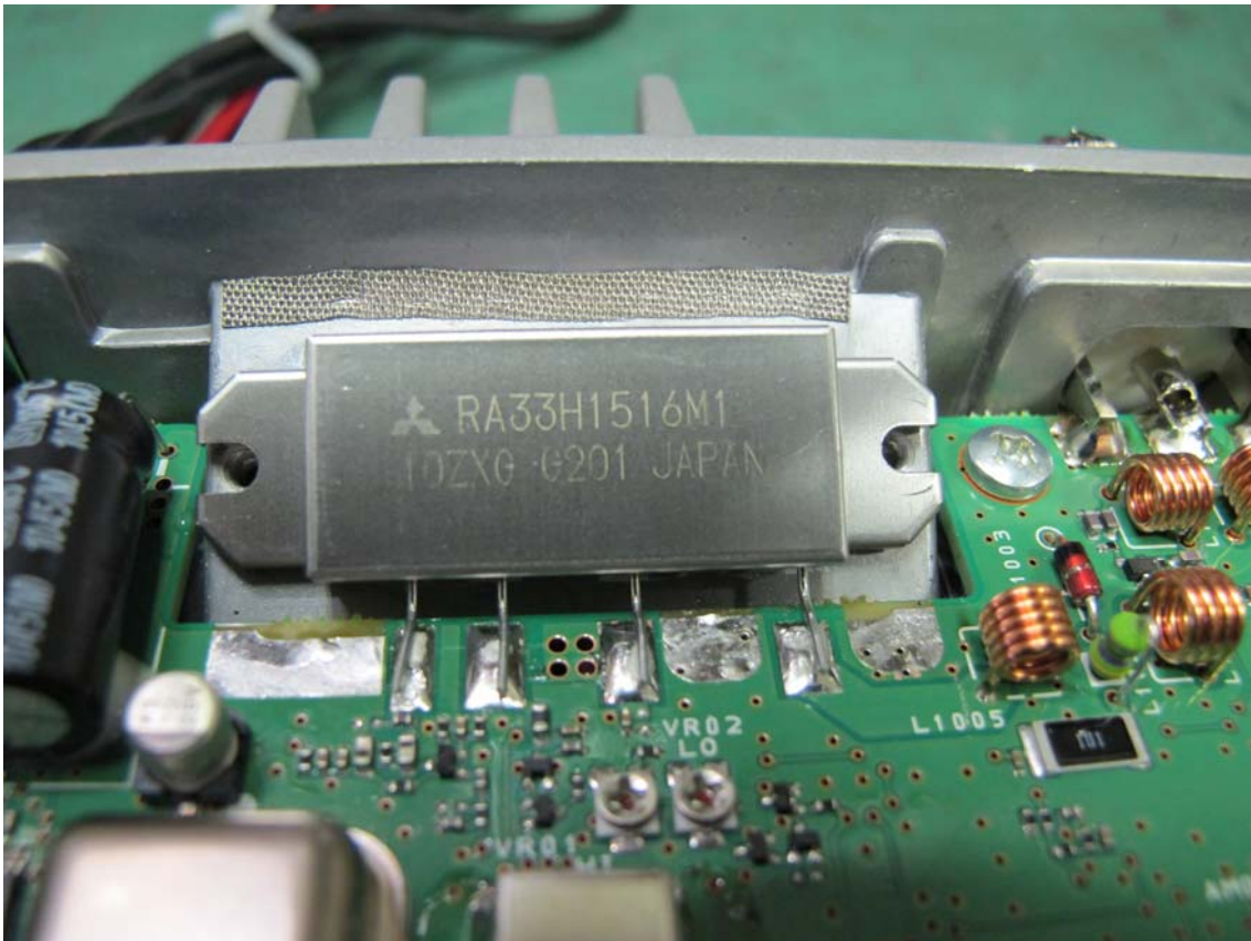
Close-up of Replacement Power Module
