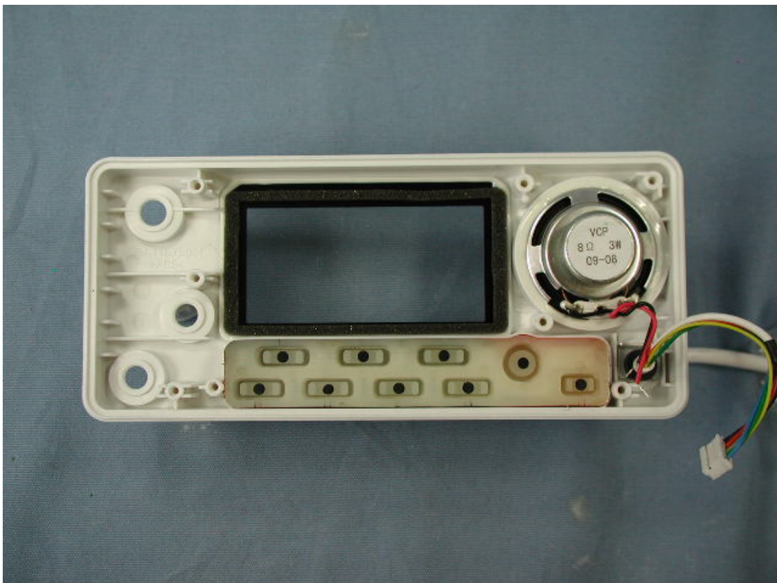
Inside of Front panel without CONT-UNIT
