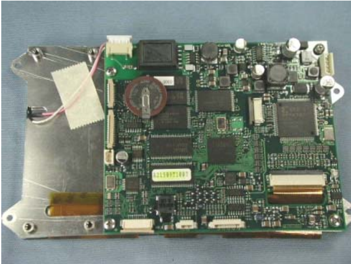
Main board side of chart plotter unit
