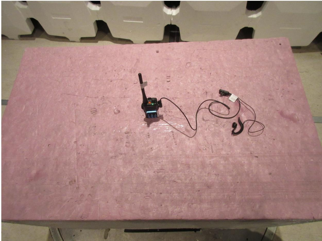
**POWERLINE CONDUCTED EMISSIONS TEST SET UP**
