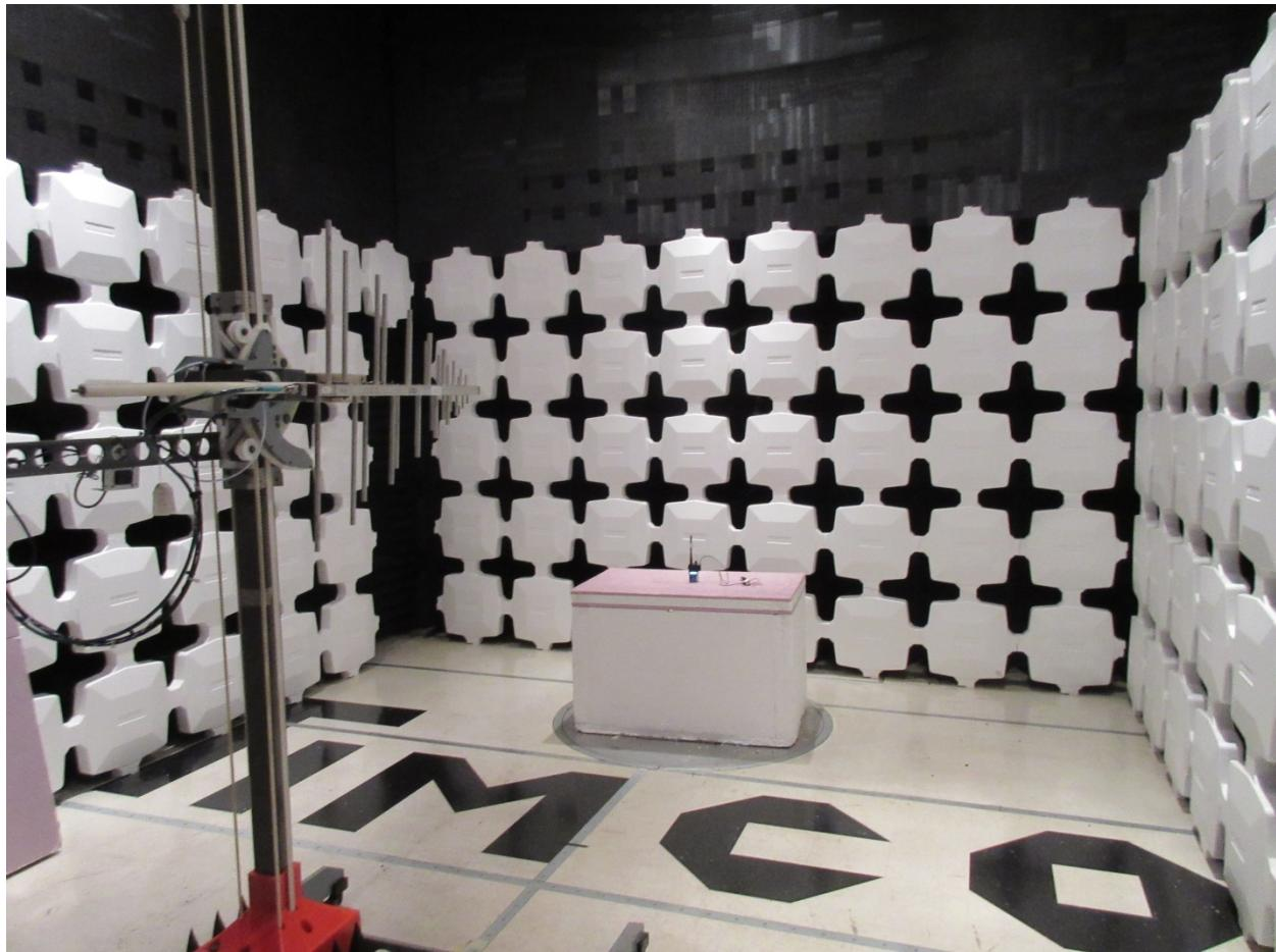
**Radiated Setup Above 1GHz**
