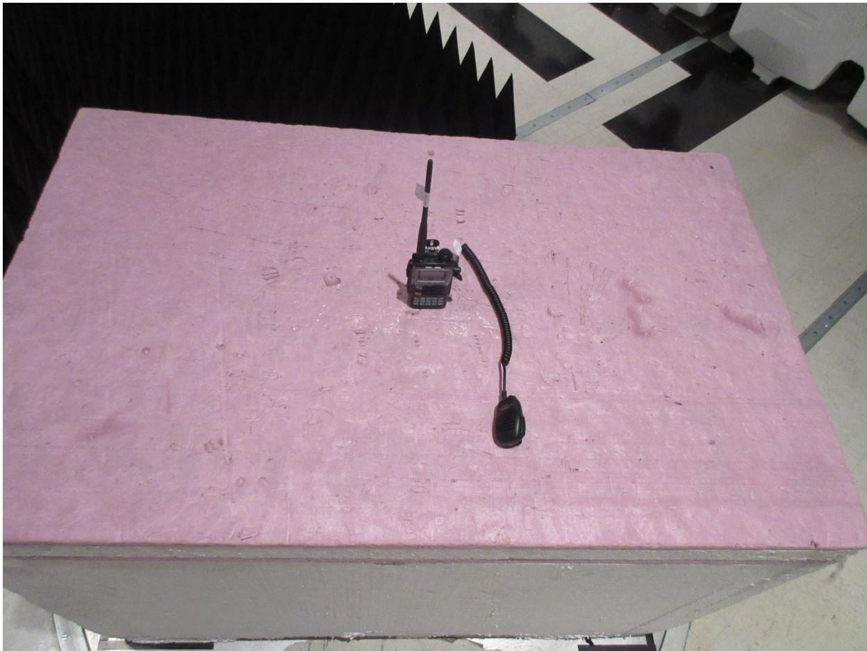
**POWERLINE CONDUCTED EMISSIONS TEST SET UP**
