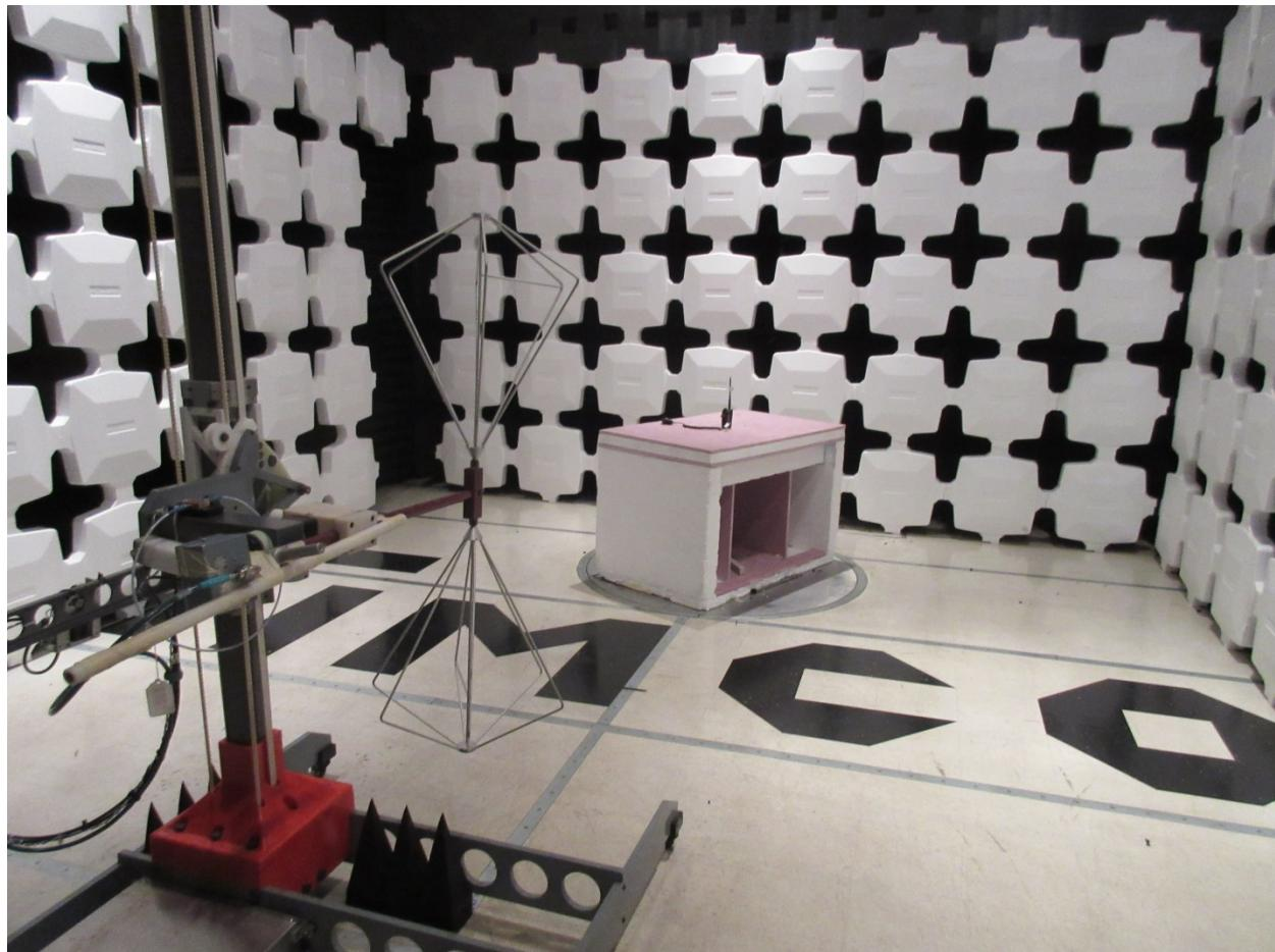
**Radiated Setup Above 1GHz**
