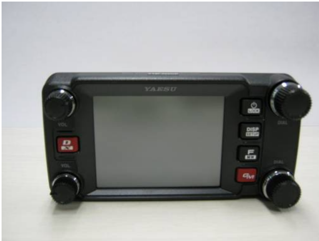
Fig.2-3 PANEL-UNIT (Front View)
