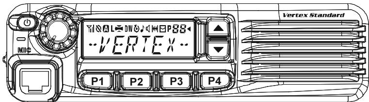
The **VX-4600** Series are full-featured FM transceivers designed for flexible mobile and base station business communications in the VHF or UHF Land Mobile bands. These transceivers are designed for reliable business communications in a wide variety of applications with a wide range of operating capability provided by their leading-edge design.
