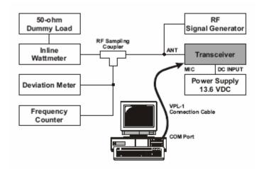
The transceiver must be programmed for use in the intended system before alignment is attempted. The RF parameters are loaded from the file during the alignment process. In order to facilitate alignment over the complete switching range of the equipment it is recommended that the channel data in the transceiver is preset as the chart below.
