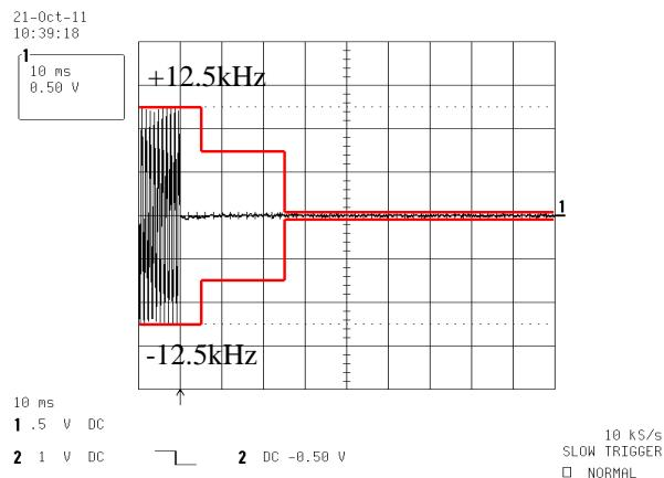
State : High Power / Authorized Bandwidth 11.25 kHz / 11K0F3E / 161.5 MHz (FCC/ RSS)/ PTT:ON -OFF
