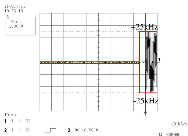
State : High Power / Authorized Bandwidth 11.25 kHz / 11K0F3E / 161.5 MHz (FCC/ RSS)/ PTT:OFF -ON
