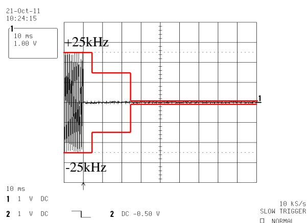
State : High Power / Authorized Bandwidth 20 kHz / 16K0F3E / 161.5 MHz (FCC/ RSS)/ PTT:ON -OFF
