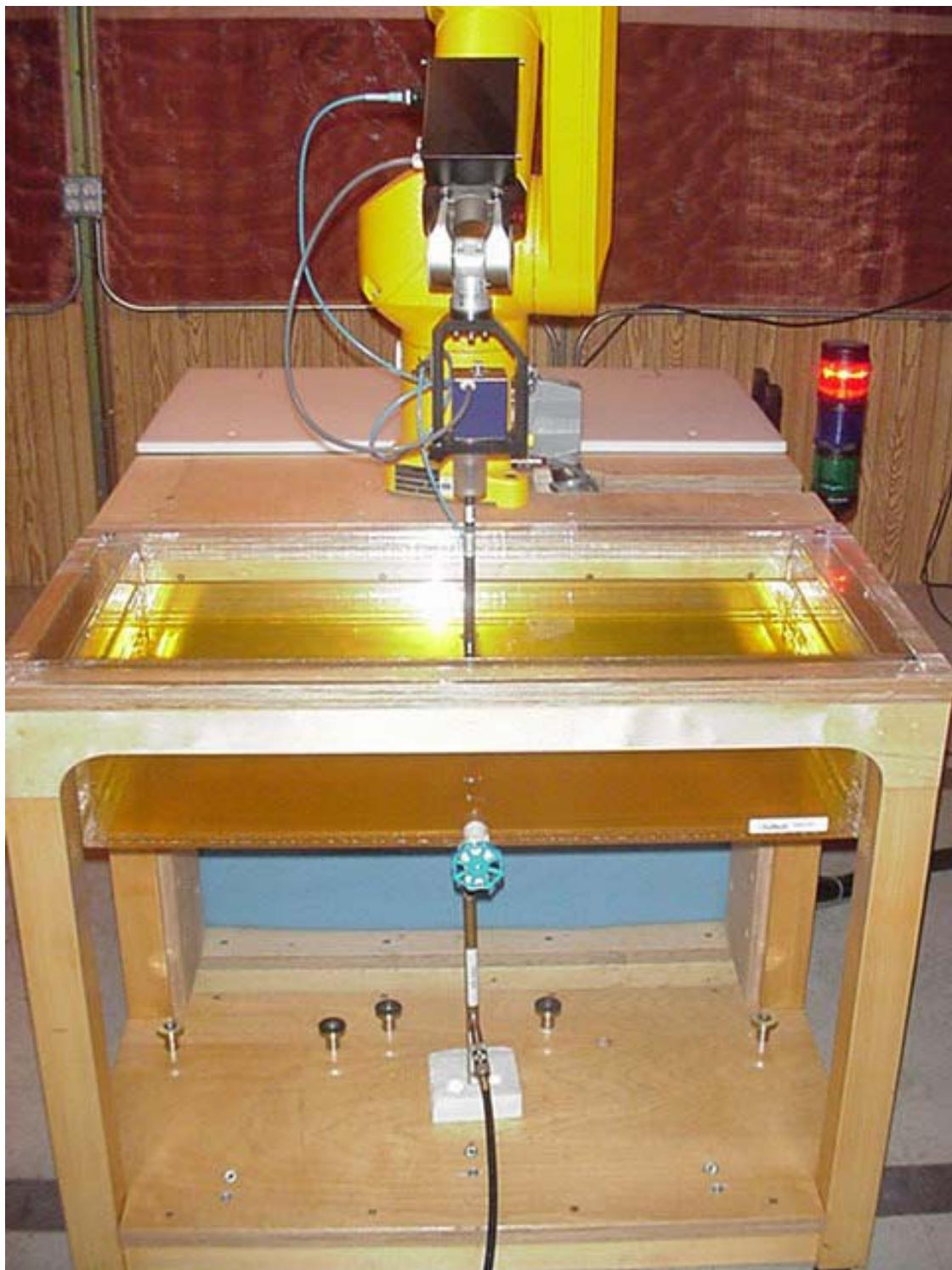
**7. 450 MHz Validation Dipole Setup**
