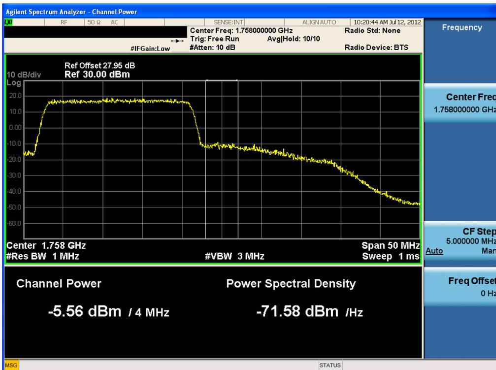
■ Low Emission Mask (LTE Band 13\_763 MHz – 775 MHz) QPSK –RB Size 50
