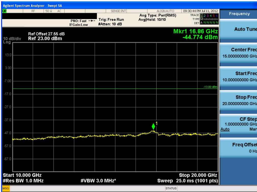
Conducted Spurious Plot (LTE Band 4\_10MHz QPSK - RB Size 1, RB Offset 49 - High Channel)-2
