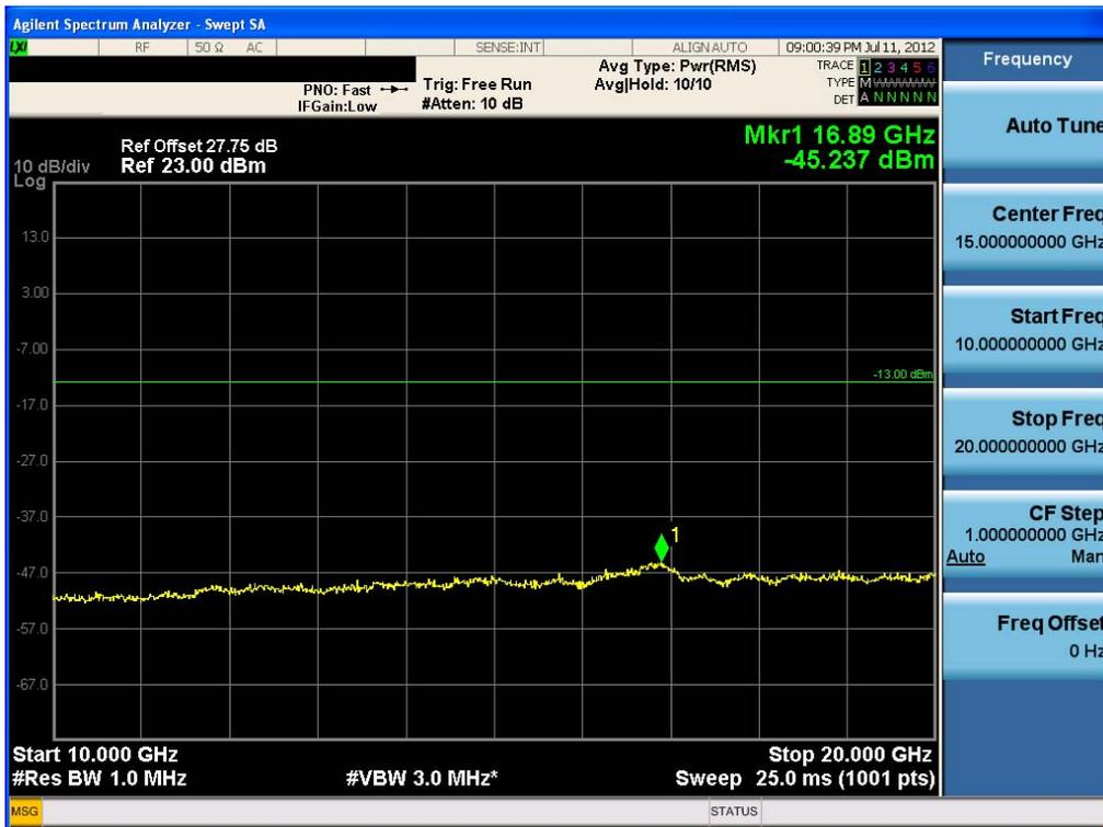
Conducted Spurious Plot (LTE Band 4\_5MHz QPSK - RB Size 1, RB Offset 24 - High Channel)-2
