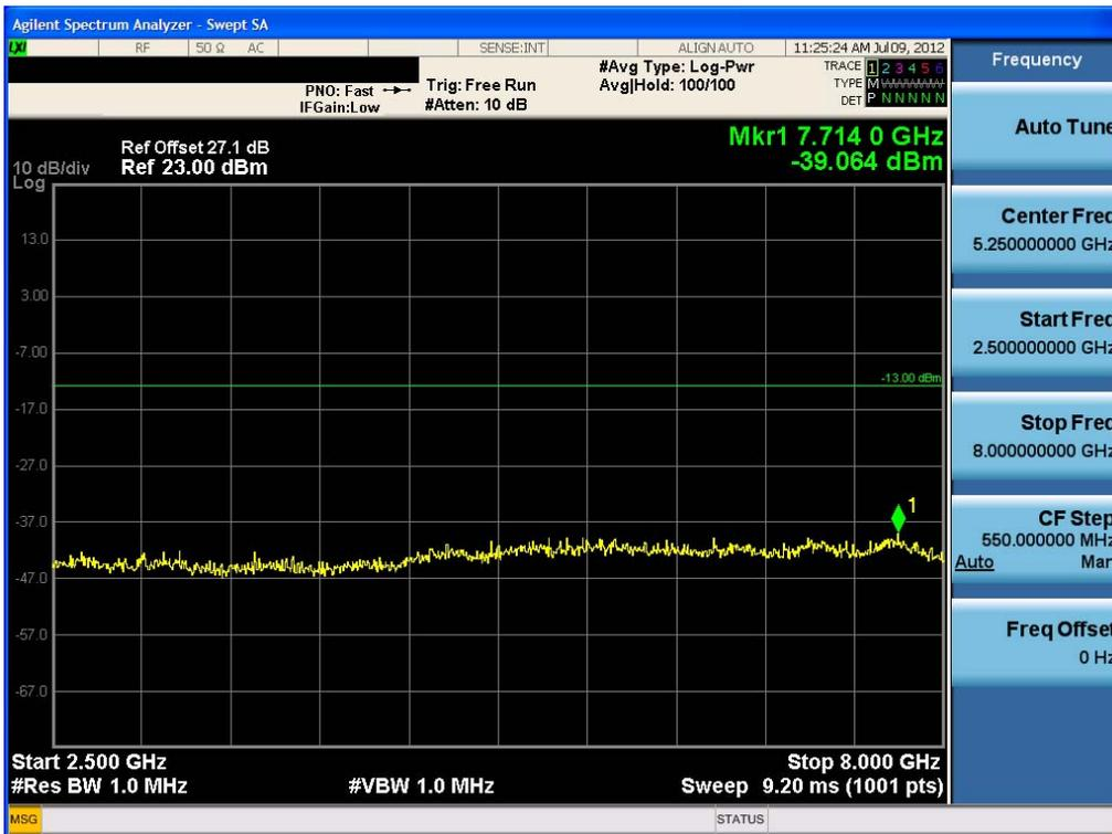
■ Conducted Spurious Emission (LTE Band 13\_QPSK – RB Size 1, RB Offset 49)-2
