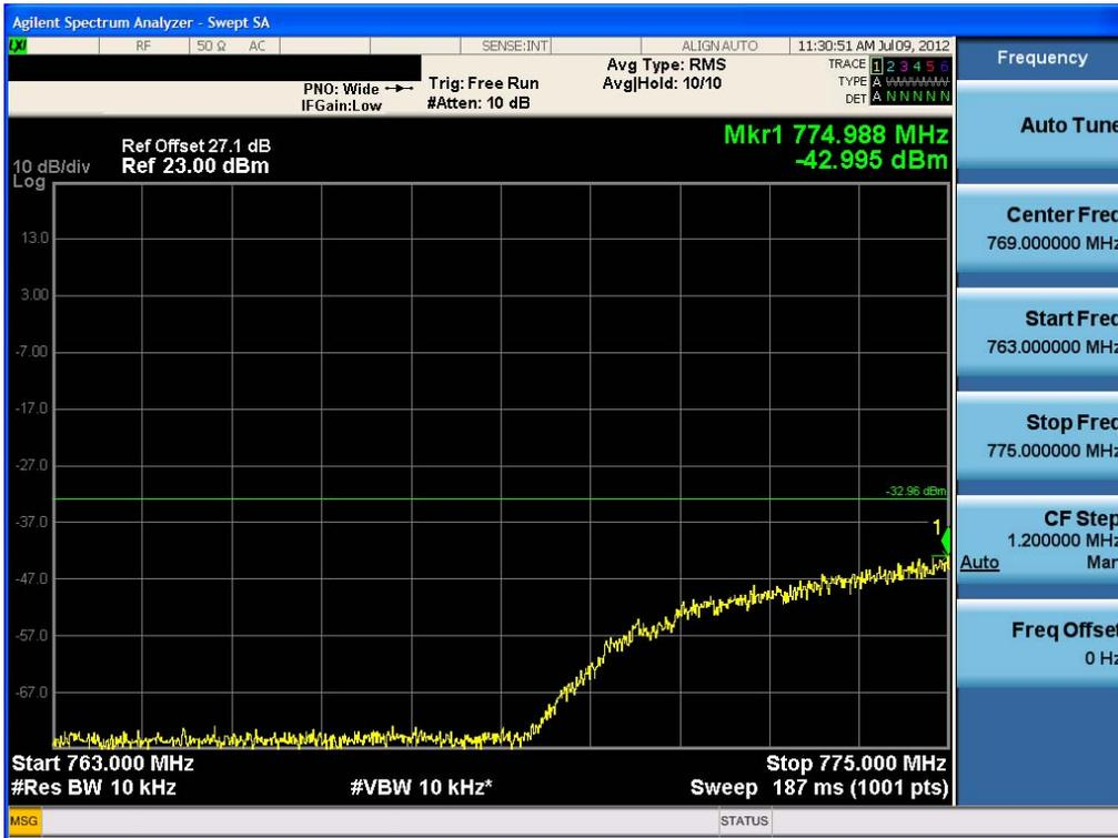
■ Upper Emission Mask (LTE Band 13\_793 MHz – 805 MHz) QPSK –RB Size 50
