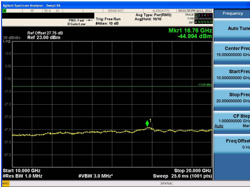
Conducted Spurious Plot (LTE Band 4\_5MHz QPSK - RB Size 1, RB Offset 0 - Mid Channel)-2
