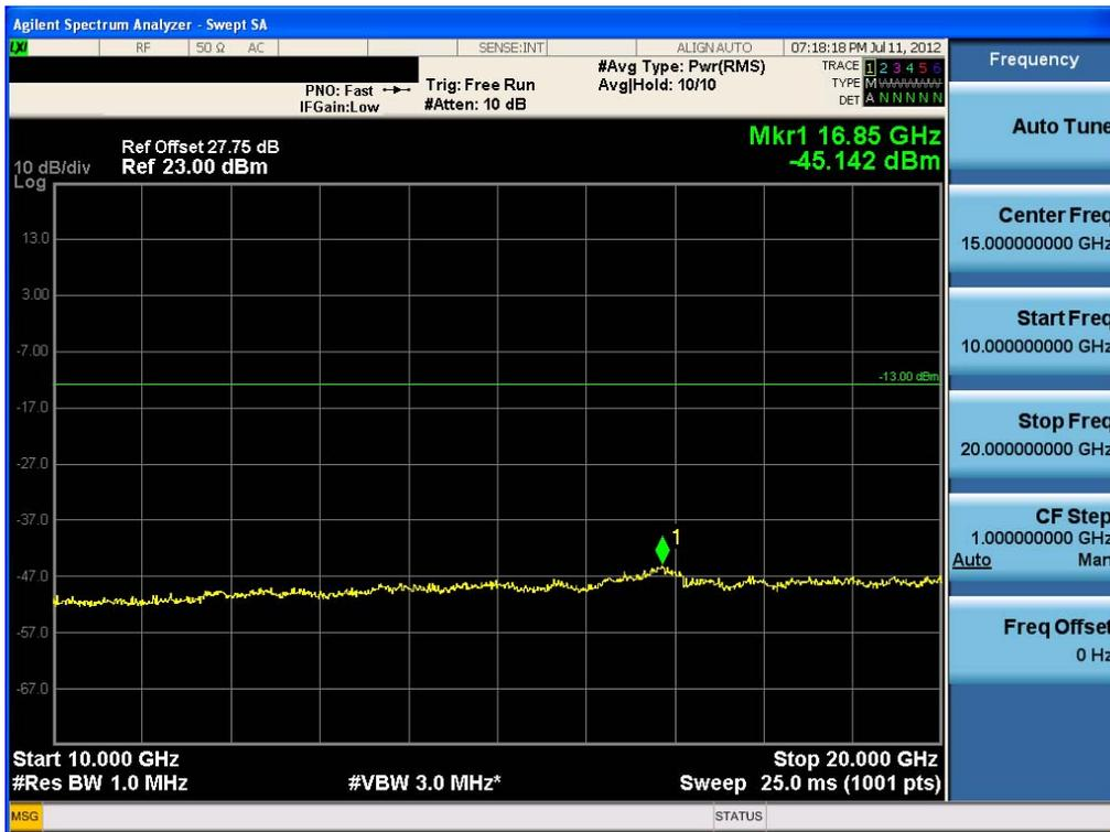
Conducted Spurious Plot (LTE Band 4\_5MHz QPSK - RB Size 1, RB Offset 24 - Low Channel)-2
