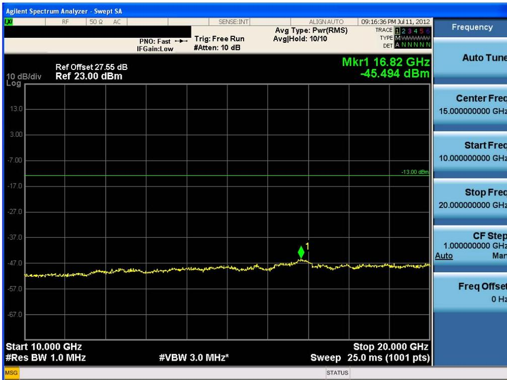
Conducted Spurious Plot (LTE Band 4\_10MHz QPSK - RB Size 1, RB Offset 0 - Mid Channel)-2
