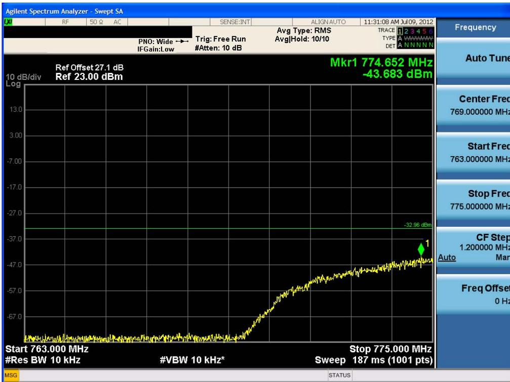
■ Upper Emission Mask (LTE Band 13\_793 MHz – 805 MHz) 16-QAM –RB Size 50
