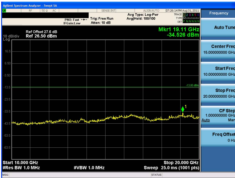
Conducted Spurious Plot (10 MHz BW, QPSK, Band 4 – Mid Channel)
