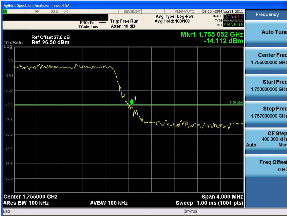
Band Edge Plot (5 MHz BW, QPSK, Band 4 – High Channel)
