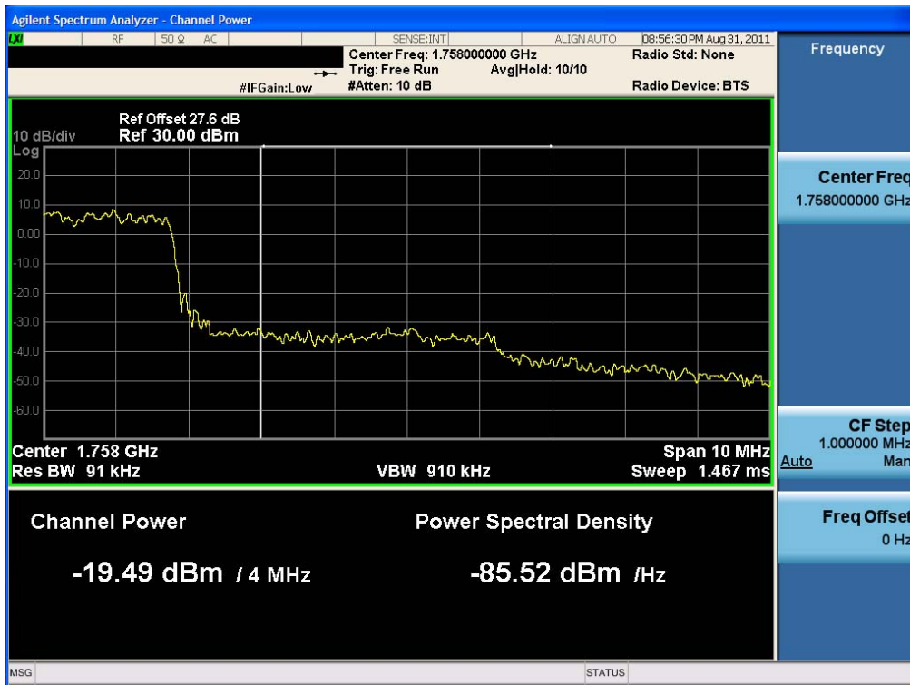
Extended Band Edge Plot (5 MHz BW, QPSK, Band 4 – High Channel)
