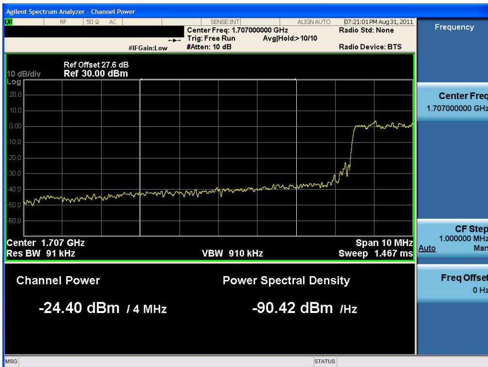
Extended Band Edge Plot (10 MHz BW, QPSK, Band 4 – Low Channel)
