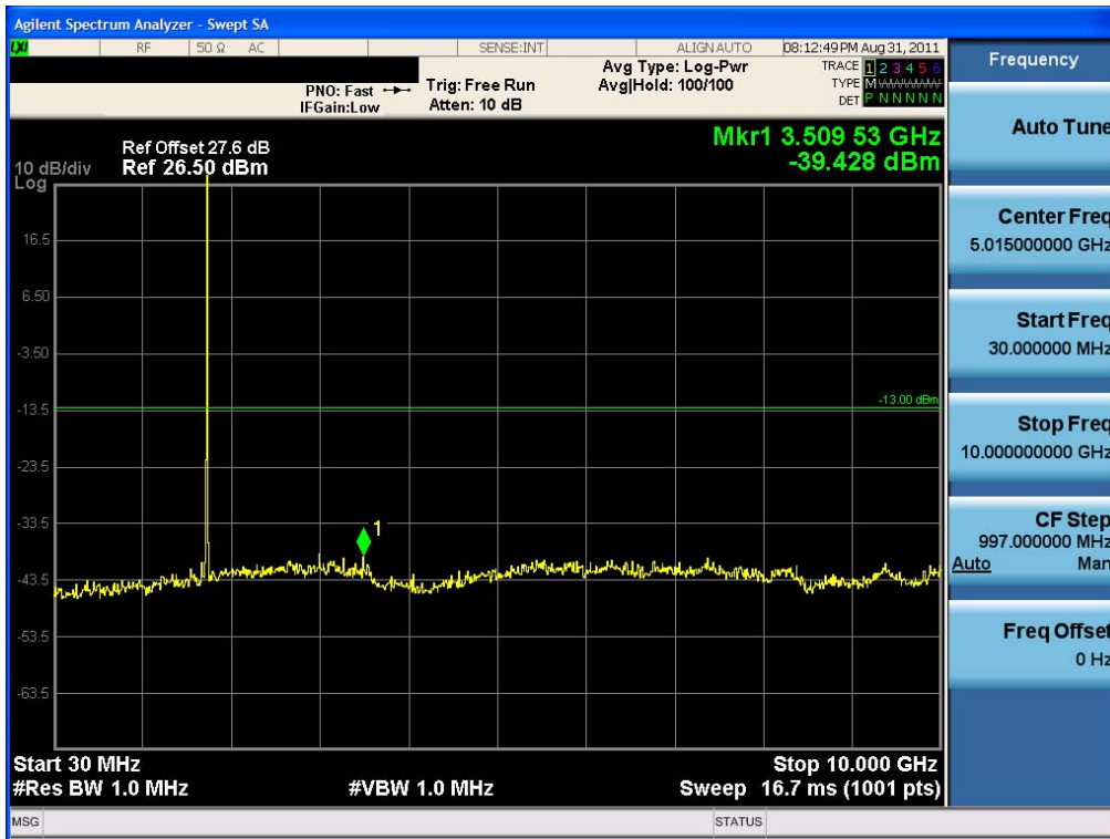
Conducted Spurious Plot (5 MHz BW, QPSK, Band 4 – High Channel)
