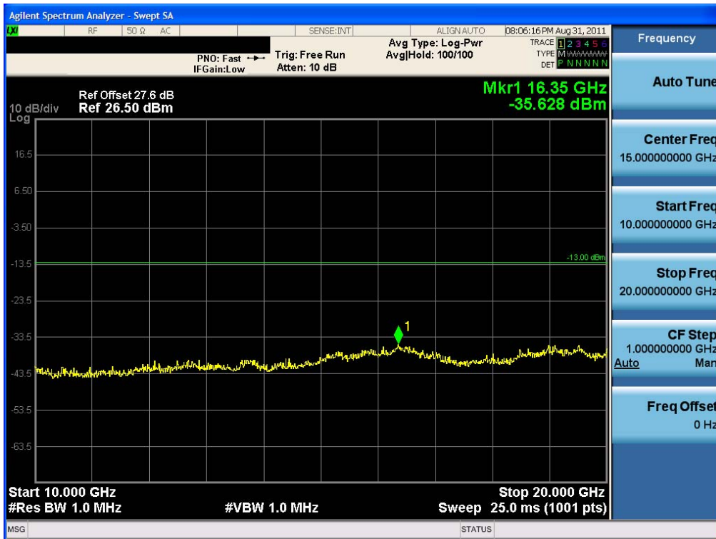
Conducted Spurious Plot (5 MHz BW, QPSK, Band 4 – Mid Channel)
