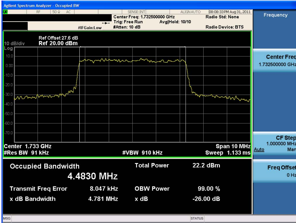
Occupied Bandwidth Plot (5 MHz BW, 16-QAM, Band 4 –Mid Channel)
