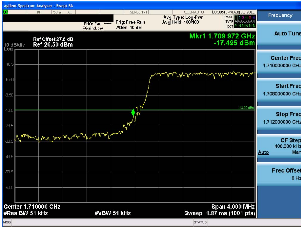
Band Edge Plot (5 MHz BW, QPSK, AWS Band – Low Channel)
