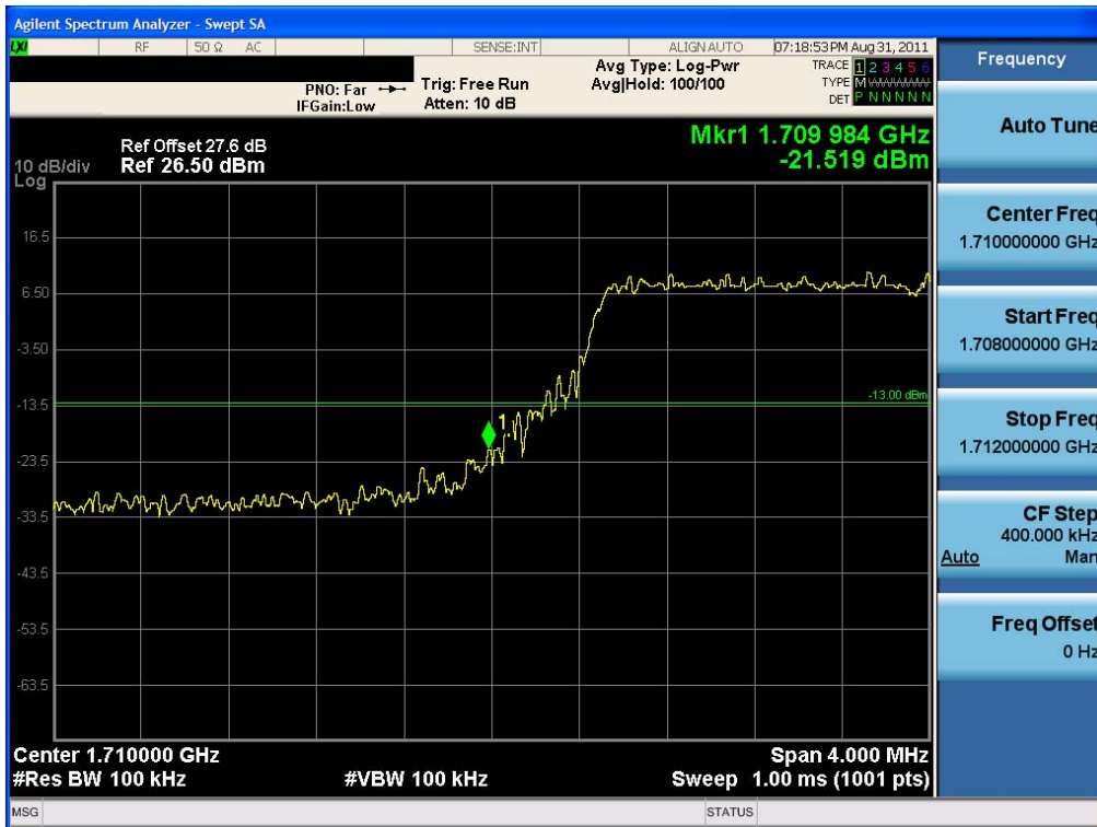
Band Edge Plot (10 MHz BW, QPSK, Band 4 – Low Channel)
