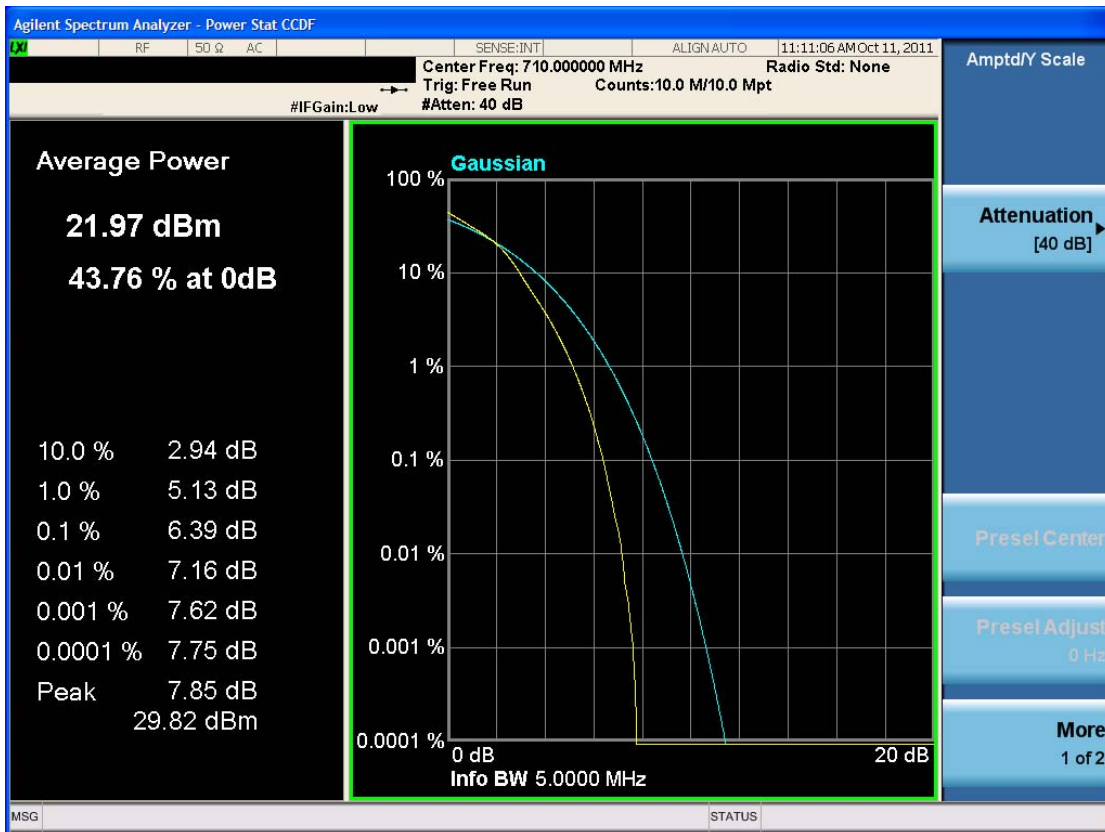
Peak-Average Ratio Plot (5 MHz BW, 16QAM, Band 17 – Mid Channel)
