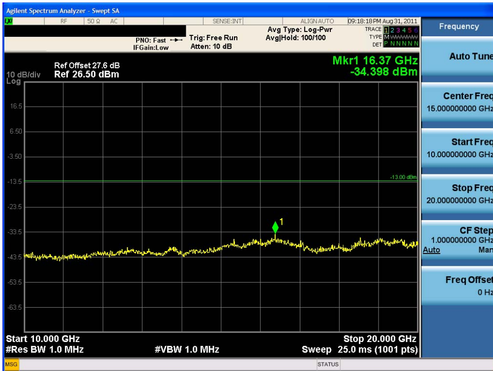
Conducted Spurious Plot (10 MHz BW, QPSK, Band 4 – Low Channel)
