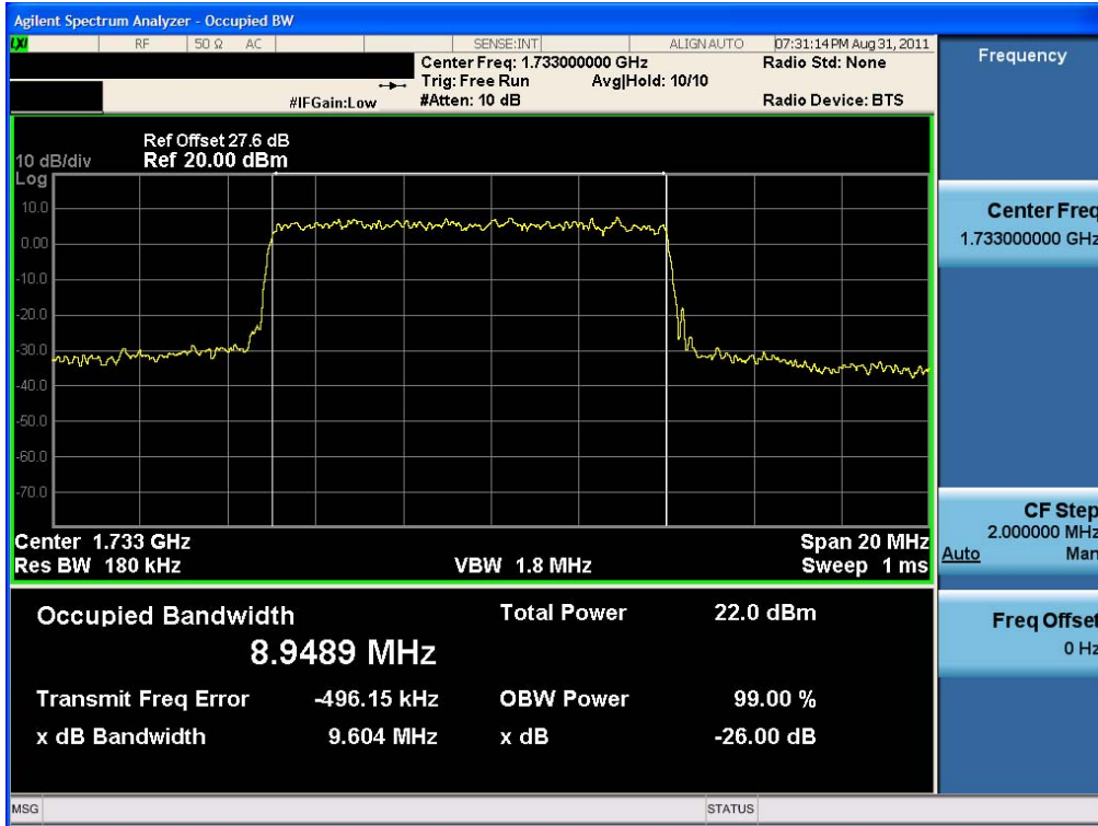
Occupied Bandwidth Plot (10 MHz BW, QPSK, Band 4 –Mid Channel)
